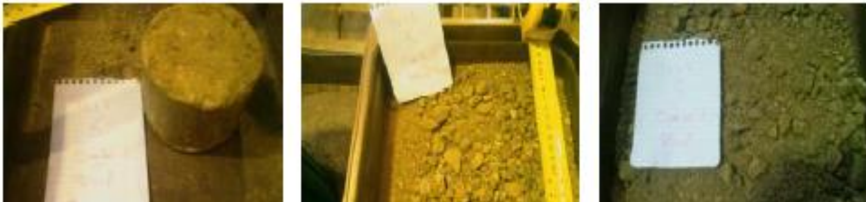
Sequential dry drops on a pressed oxide ore
