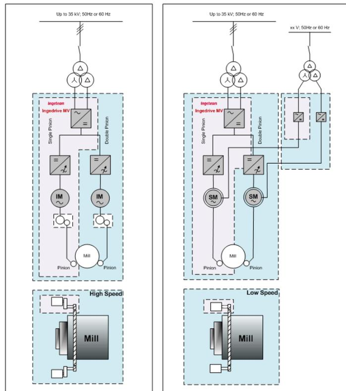
Figure 1 – General overview of the high speed and low speed drive system solutions for gear driven mills (single or dual pinion) (Ingeteam).
