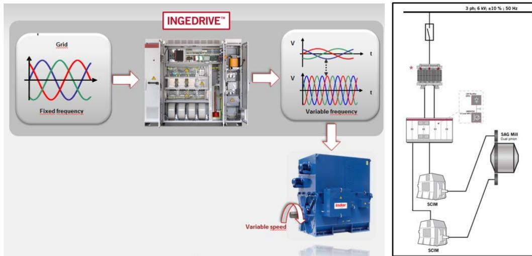
Figure 6 – Speed regulation and load sharing by Ingedrive VSDs (Ingeteam)
