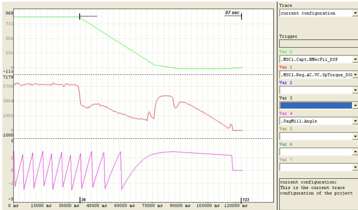
Figure 8 – Controlled Stop sequence in the Rudnik Alexandrovskiy project (Ingeteam VSD data)
