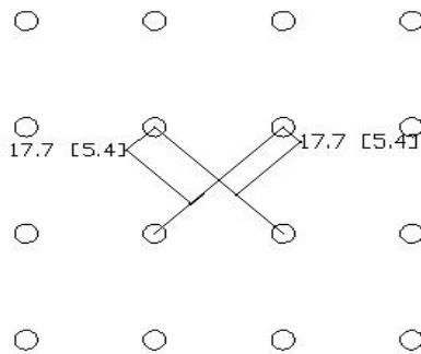
Figure 6 – Furthest distance from a blasthole for a 7.6 x 7.6 meter square pattern
