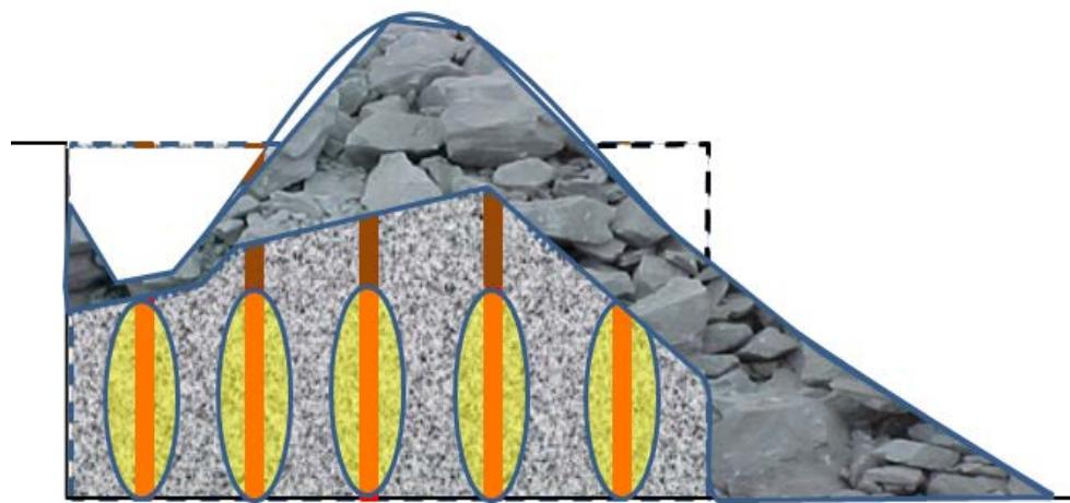
Figure 8 – Representation of fragmentation zones within a blast
