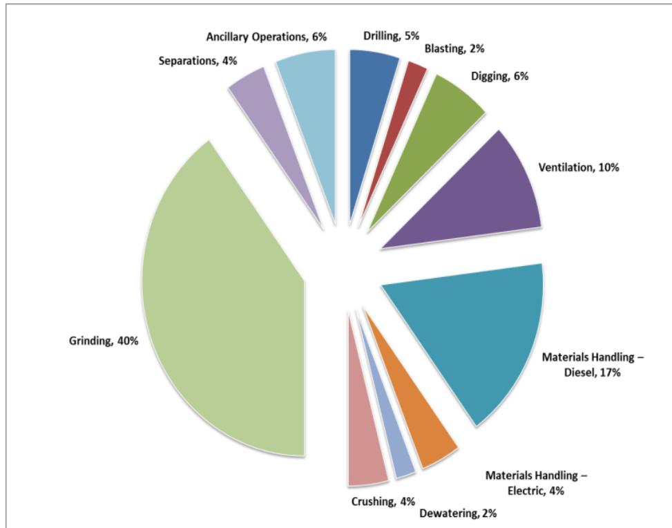
Figure 2 – Distribution of energy consumption (DOE, 2007) at a hard rock mining facility
