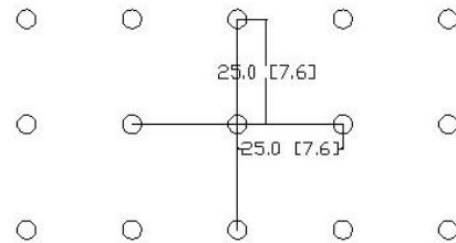
Figure 4 – Arrangement of blastholes for square pattern
