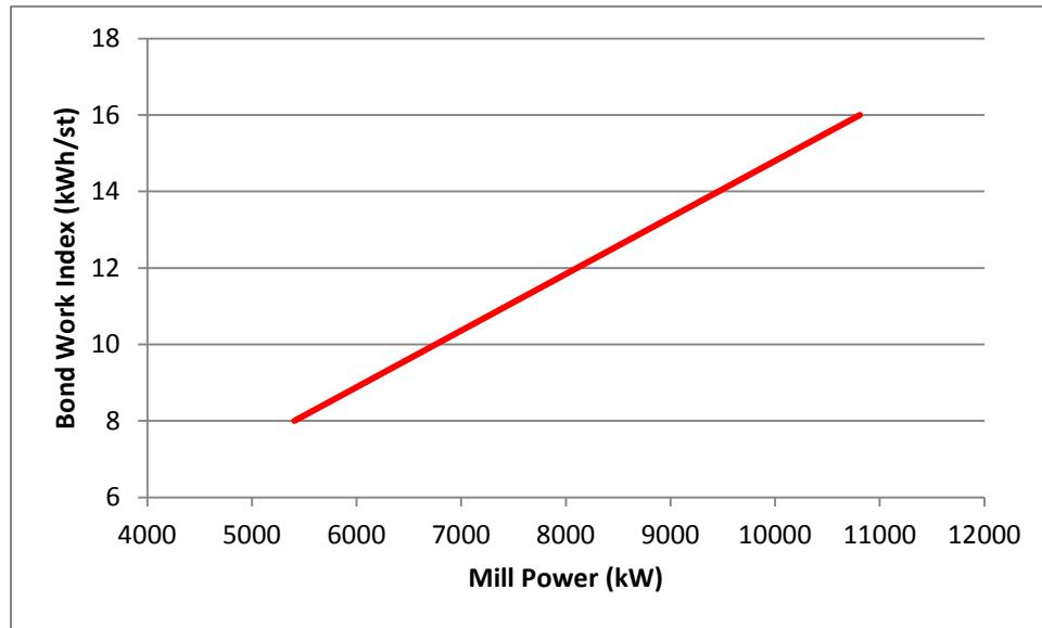
Figure 1 – Effect of mill power on a SAG mill by the change in Word Index parameter only
