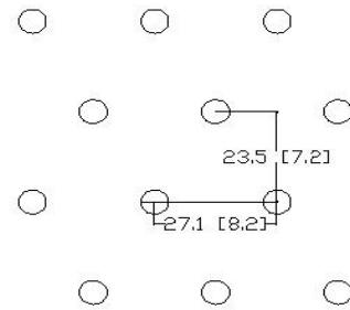
Figure 5 – Arrangement of blastholes for staggered equilateral pattern
