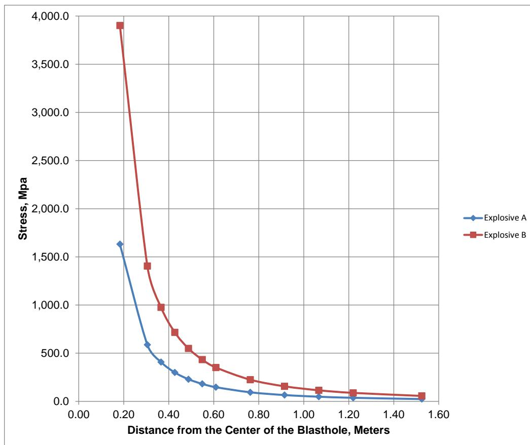
Figure 3 – Effect of distance from a blasthole on stress
