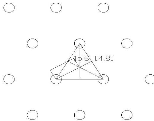
Figure 7 – Furthest distance from a blasthole for a 7.1 x 8.2 meter staggered equilateral pattern
