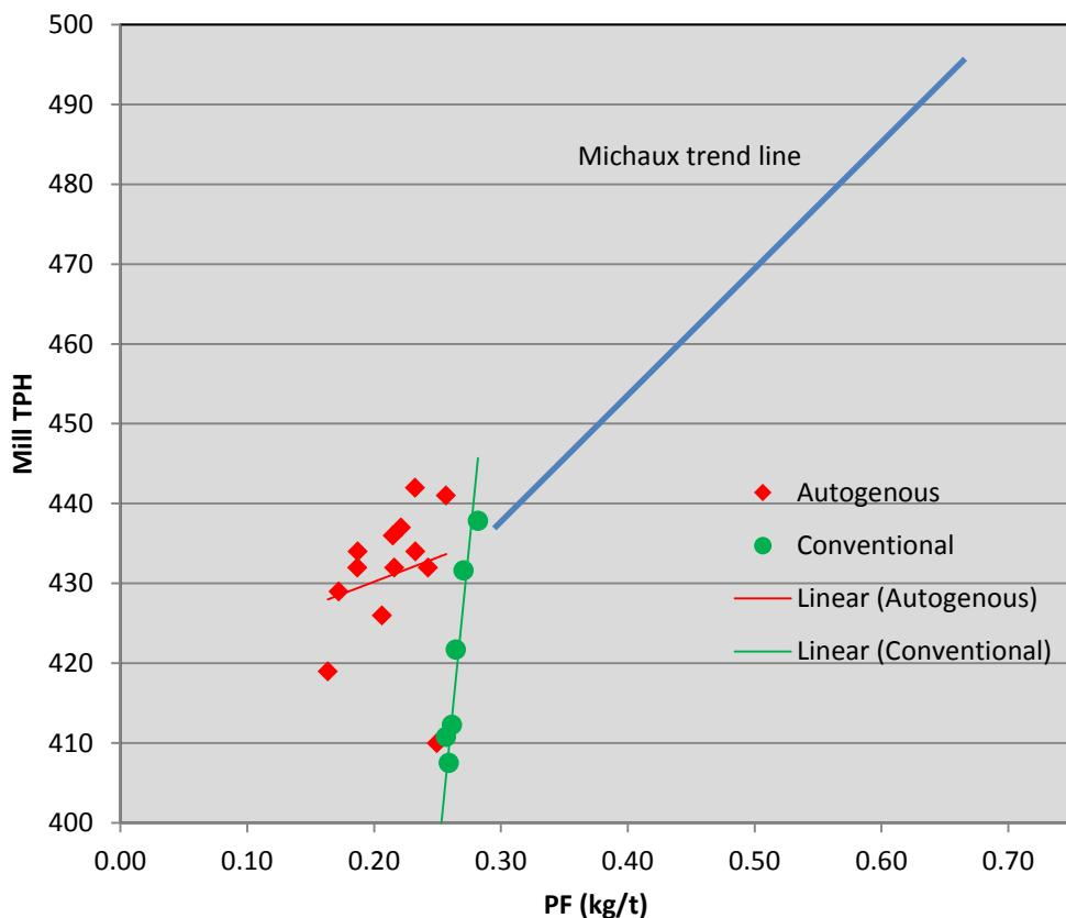
Figure 10 – Mill tons per hour vs. powder factor for conventional and autogenous grinding compared to the trend line from laboratory study by Michaux
