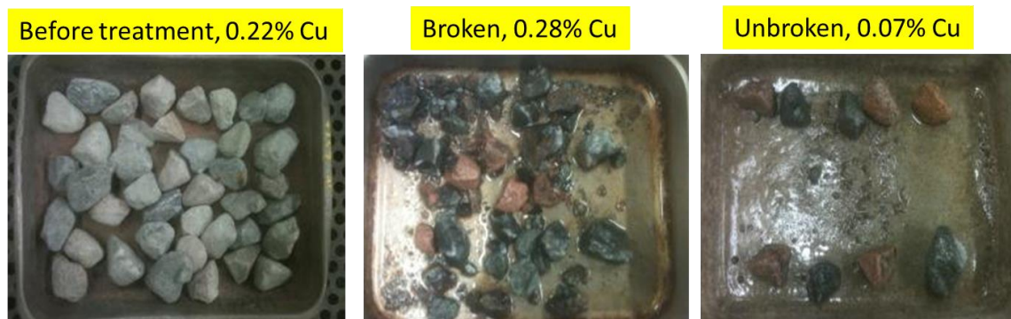
Figure 3 – SAG mill pebbles (31.5-37.5 mm) treated by high voltage pulses and separated into two groups for assay
