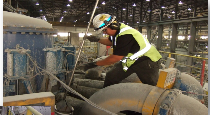
Individual cyclone overflow sampling for validation /calibration campaign
