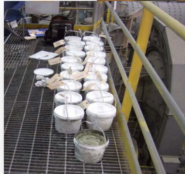
Individual cyclone overflow sampling for validation /calibration campaign
