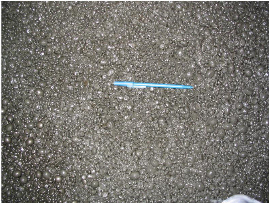
Figure 3: Picture of a 100% Millpebs charge in a regrind ball mill
