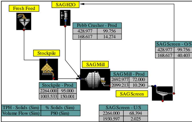
Figure 5. Case Study 2 – SABC circuit flowsheet – pre-feasibility design study to size SAG mill with JKSimMet.
