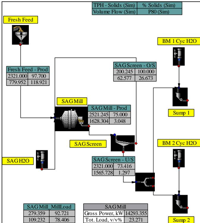
Figure 1. Case Study 1 – Existing SAG circuit flowsheet – original circuit as modelled with JKSimMet.
