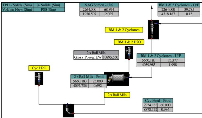
Figure 6. Case Study 2 – Ball mill circuit flowsheet – pre-feasibility design study to size SABC circuit ball mills with JKSimMet.
