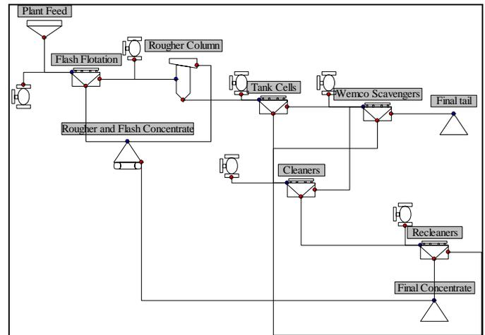
Figure 7. Kanowna Belle Gold Mine flotation circuit flowsheet.
