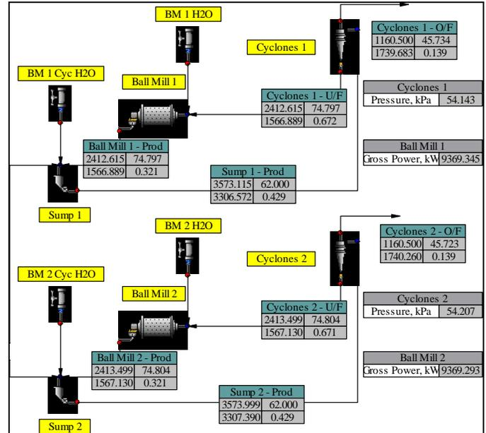
Figure 2. Case Study 1 – Ball mill circuit flowsheet – original circuit as modelled with JKSimMet.
