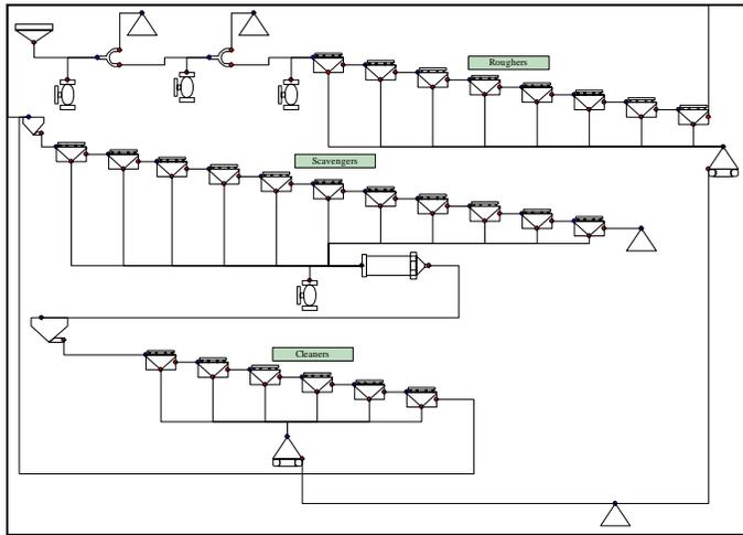
Figure 8. Century Zinc flotation circuit partial flowsheet.
