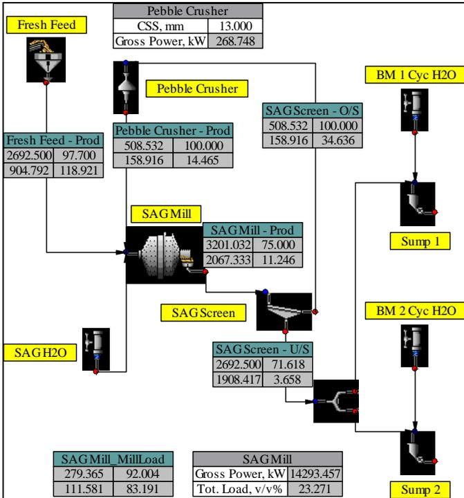
Figure 3. Case Study 1 – SAG mill circuit with pebble crusher added.
