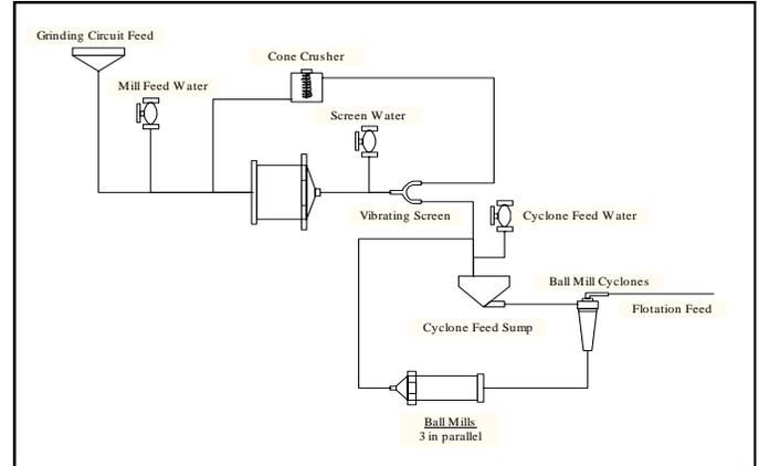
Figure 9. Laguna Seca grinding circuit flowsheet.
