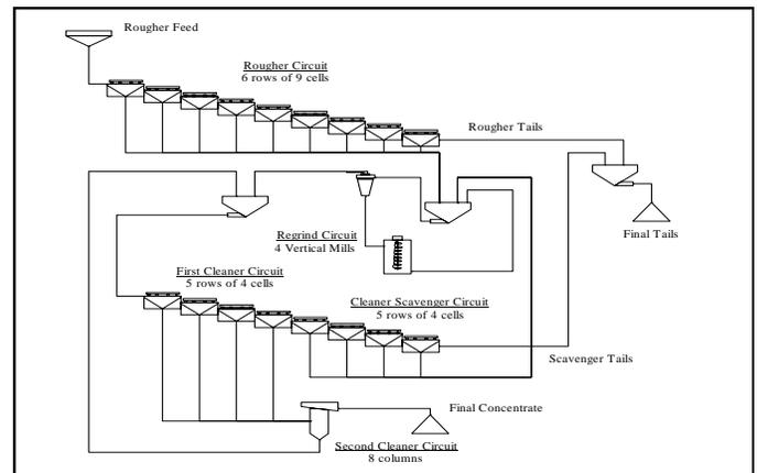
Figure 10. Laguna Seca flotation circuit flowsheet.
