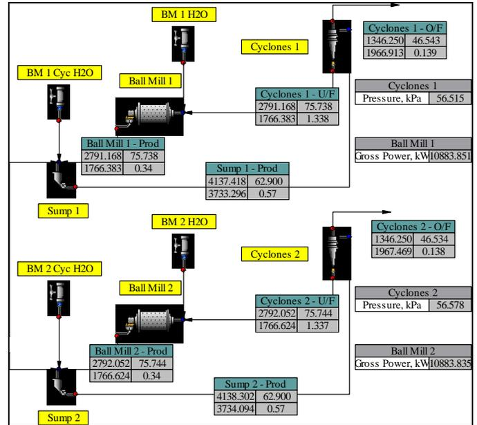
Figure 4. Case Study 1 – Ball mill circuit after pebble crusher added and ball mill optimized by adding smaller balls and increasing ball charge.
