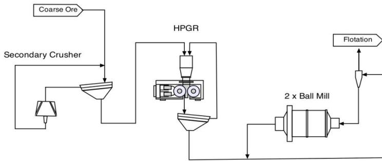
Figure 3 - HPGR ball mill circuit
