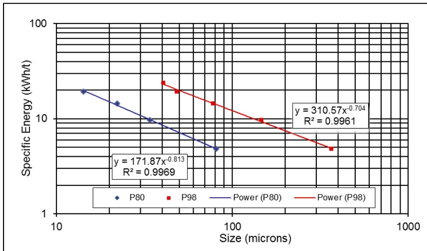
Figure 7 - Stirred mill signature plot
