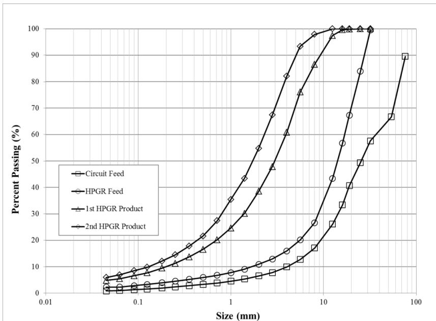
Figure 6 – HPGR feed and products particle size distribution
