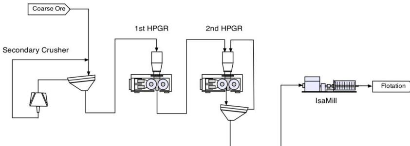
Figure 4 - HPGR - stirred mill circuit
