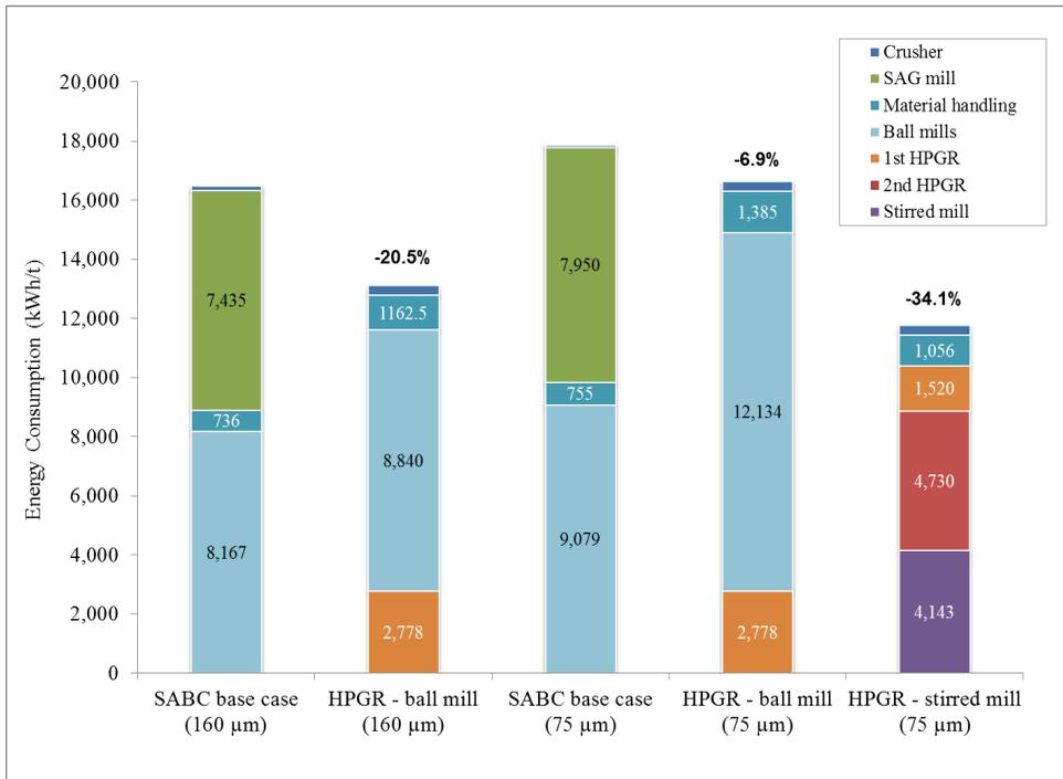
Figure 8 - Comparison of total circuit energy requirement
