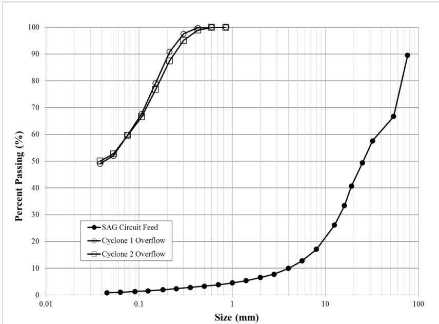
Figure 5 - Particle size distributions of plant samples
