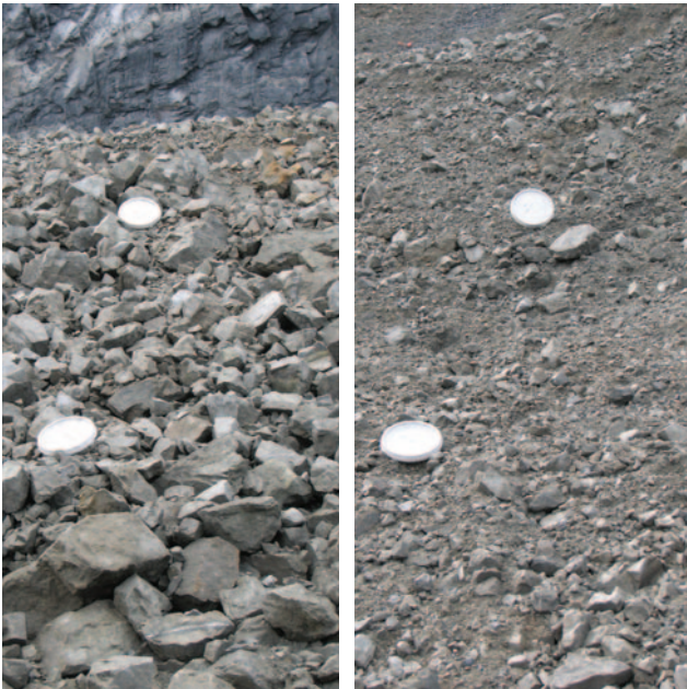
Antamina's harder copper-zinc ore before and after the mine-to-mill optimization
