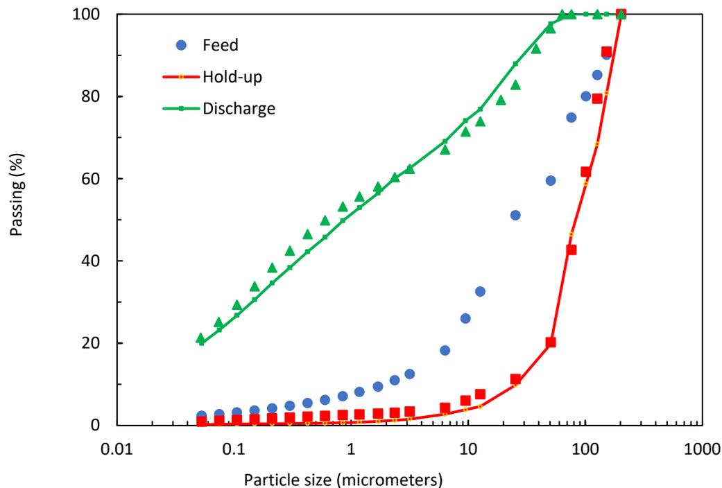
Figure 8—Comparison of measured (symbols) and predicted size distributions (lines) from milling of copper ore in a 6' x 2' pilot-scale AG mill (Carvalho and Tavares, 2014)
