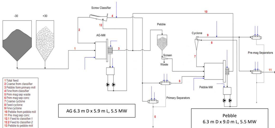
Figure 2—LKAB Magnetite AG milling circuit
