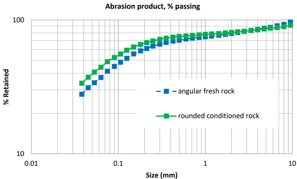
Figure 11—An example of the abrasion appearance function
