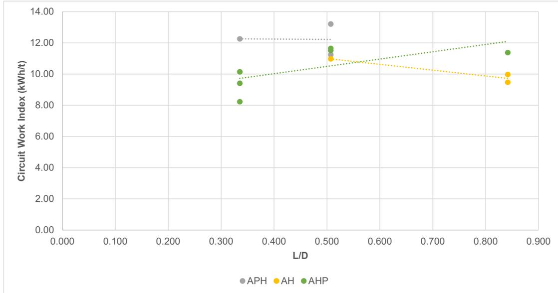
Figure 6—Impact of L/D on Circuit Operating Work Index
