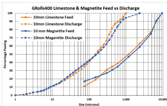
Fig. 7. GRolls® comparison Limestone vs Magnetite Feed.
