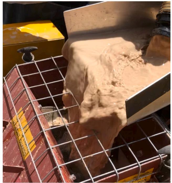
Fig. 14. GRolls® Wet 33 % solids (w/w) slurry < 3 mm limestone feed material.
