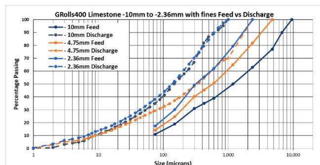
Fig. 10. GRolls®  $<10 \text{ mm}$  to  $< 2.36 \text{ mm}$  feed comparisons.
