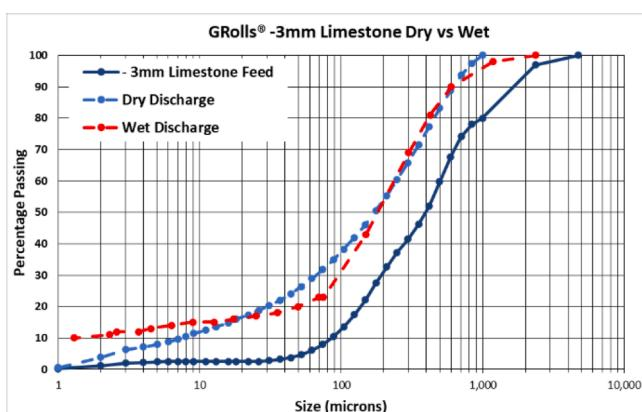
Fig. 15. Gradings of GRolls® dry vs wet 33% solids (ww) slurry test.
