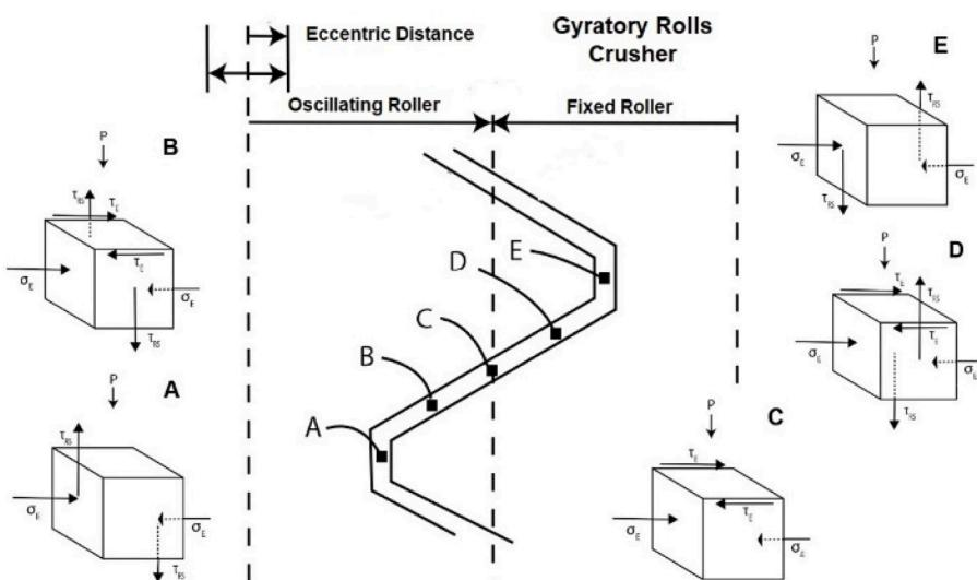
Fig. 2. GRolls® Crushing Chamber Loads.
