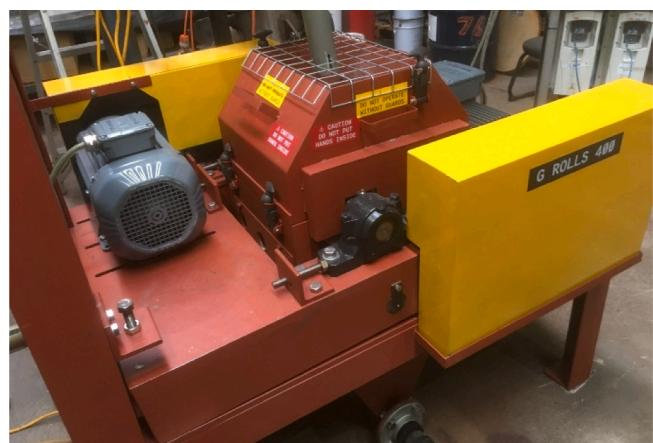
Fig. 5. Laboratory scale GRolls® GRolls400 unit.
