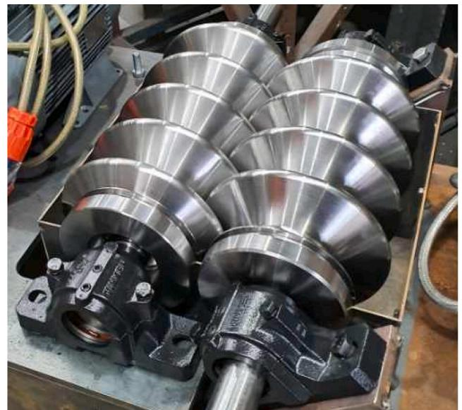
Fig. 4. Roller configuration for GRolls®.
