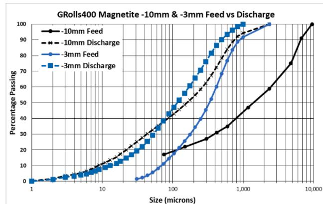
Fig. 8. GRolls® Magnetite  $< 10 \text{ mm}$  vs  $< 3 \text{ mm}$  comparison.
