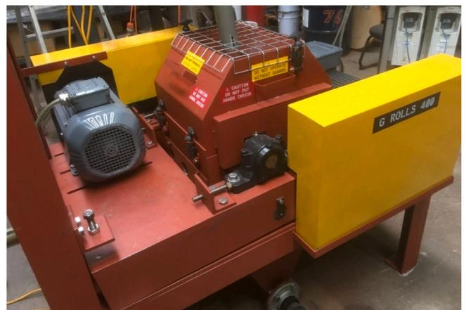
Fig. 5. Laboratory scale GRolls® GRolls400 unit.
