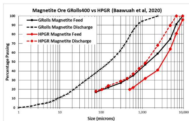
Fig. 9. Magnetite Ore Comparison GRolls® vs HPGR.
