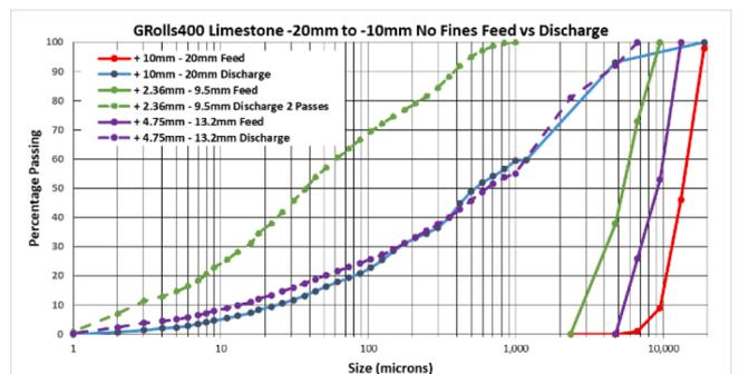
Fig. 11. GRolls® <20 mm to < 10 mm feed comparisons.
