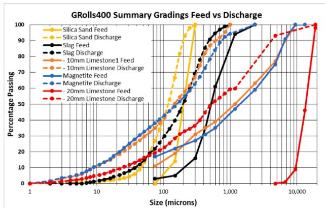
Fig. 6. GRolls® Gradings Summary Feed vs Discharge.
