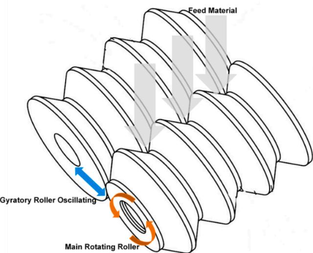
Fig. 3. Concept Design of GRolls®.
