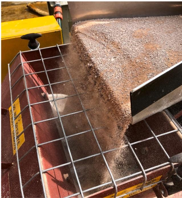
Fig. 13. GRolls® Dry < 3 mm limestone feed material.
