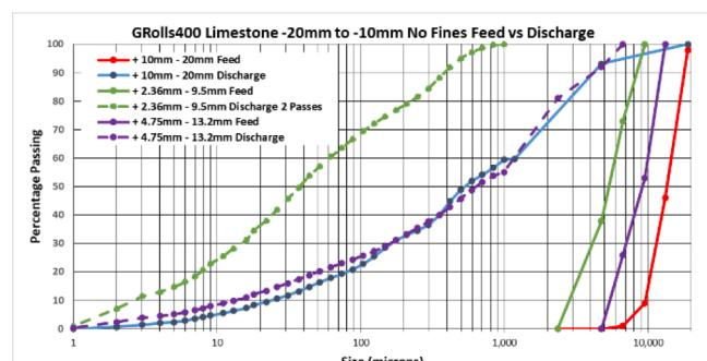
Fig. 11. GRolls®  $<20 \text{ mm}$  to  $< 10 \text{ mm}$  feed comparisons.
