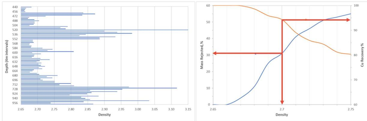
FIG 7 - Density variation down the drill hole (left) and resulting Cu recovery and mass rejection (right)
