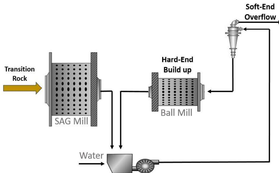
**FIG 4** – Typical SAG – ball milling circuit configuration.
