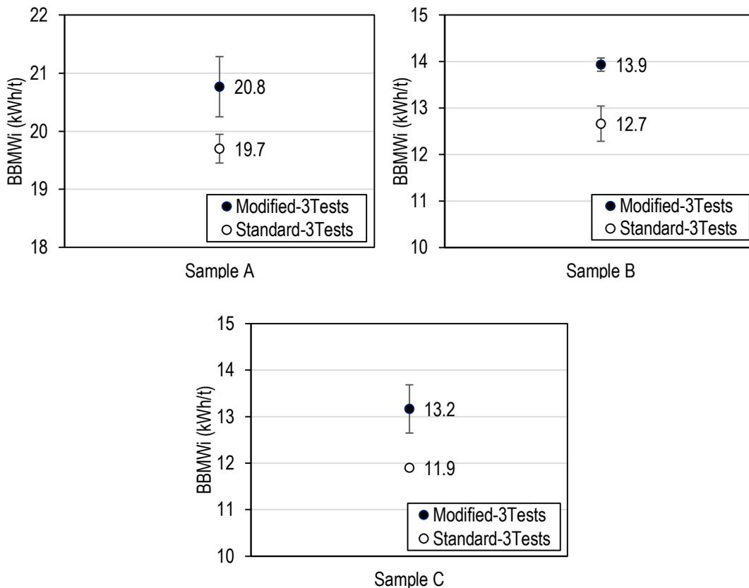
**FIG 6** – Comparison of standard and modified BBMWi values.
