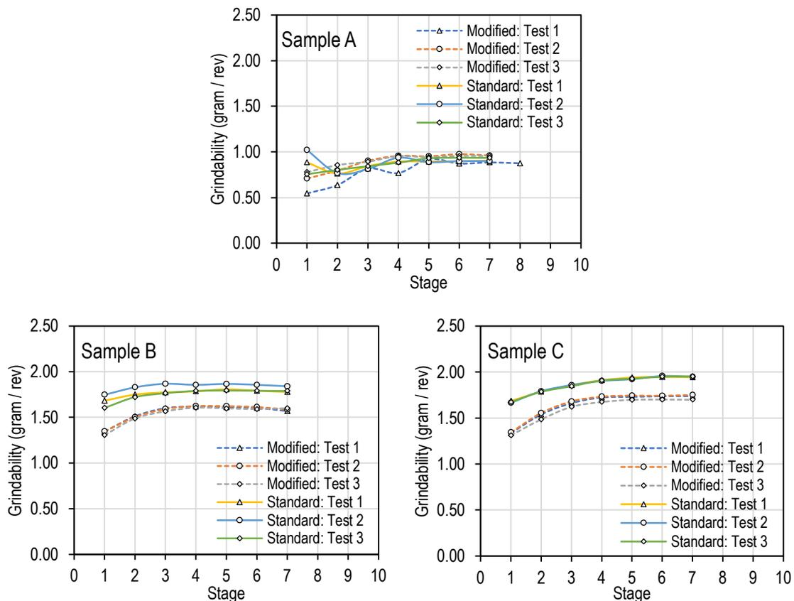
**FIG 7 – Grindability rate per stage for all Bond ball mill tests.**
