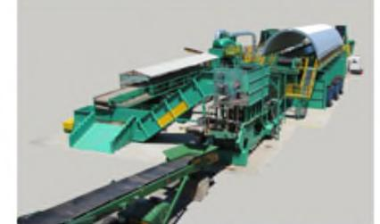
On-line sensing and separation of coarse streams
