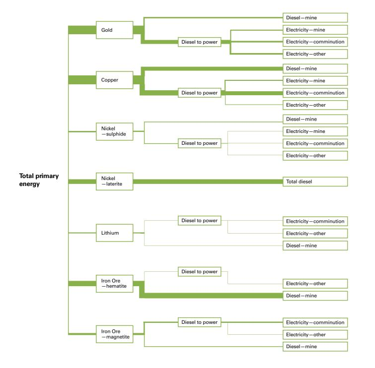
The Sankey diagram shown above provides an indication of energy flows in the industry for the commodities under investigation and shows primary energy and final energy.
