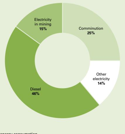
Figure 3 – Split of energy consumption across the mining industry
