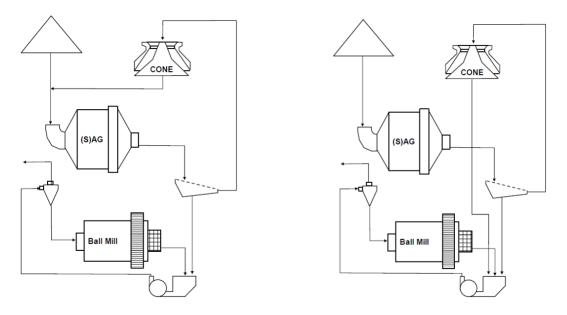
Figure 5 (left side). Pebble crushing by Cone crusher, product back to (S)AG. Figure 6 (right side). Pebble crushing by cone, product forward to downstream ball mill discharge pump sump.
