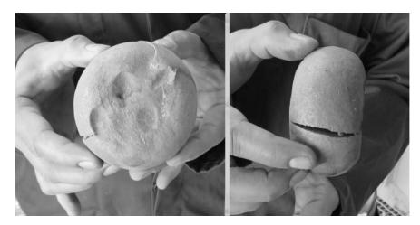
Figure 1. Example of Aerofall ball retrieved after HPGR passage, cracked and dented by HPGR rolls.
