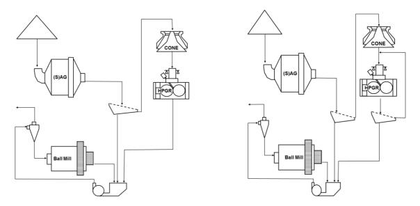
Figure 7 (left side). Pebble crushing by cone and subsequent HPGR in open circuit, product forwarded to downstream ball mill discharge pump sump.
