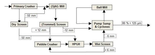
Figure 3. Penasquito Flow Sheet around HPGR.
