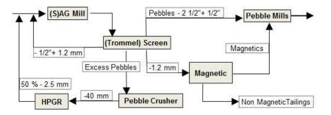
Figure 2. Empire Concentrator Flow Sheet around HPGR. Lines 22-24.
