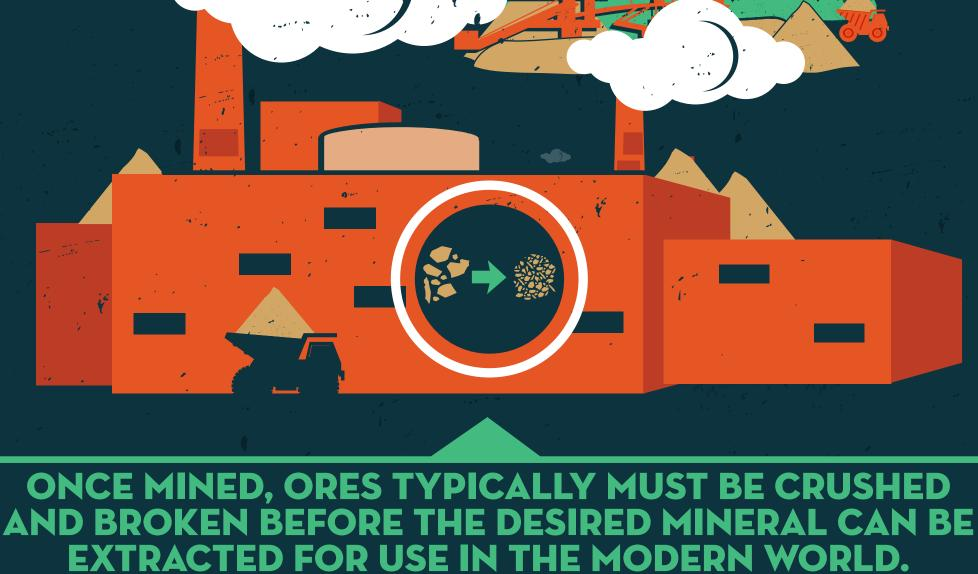
THIS PROCESS OF GRINDING AND **GRINDING & CRUSHING CRUSHING ORE - COMMINUTION - REQUIRES HUGE AMOUNTS OF COSTLY POWER.**
