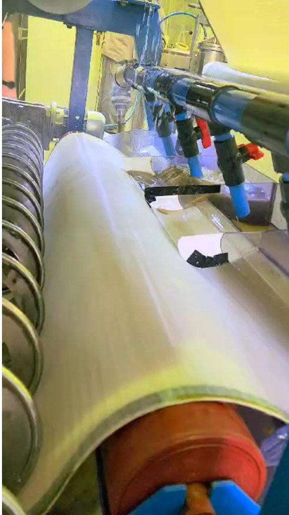
Slack Screen Primary Dewatering
