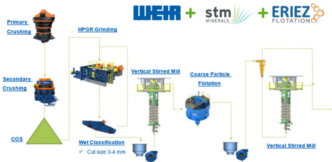
Figure 1 – Transformational Flowsheet - Weir/STM/Eriez Alliance
