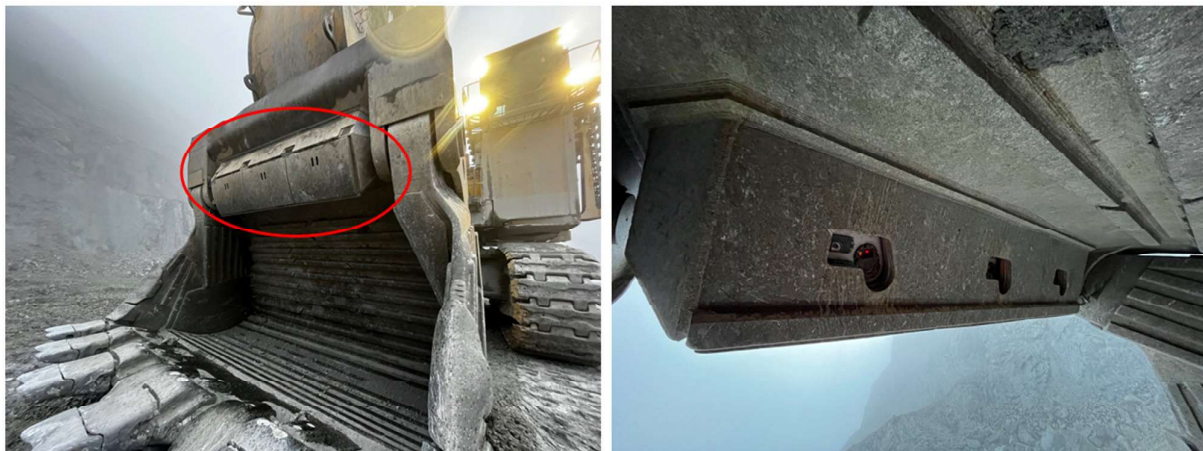
FIG 9 – Three head system on the shovels at Red Chris showing the outer armour and the inner laser, XRF emitter and X-ray receiver.
