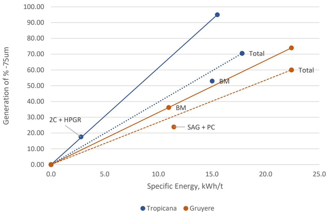
Figure 9—SSE75 Comparison by Stage
