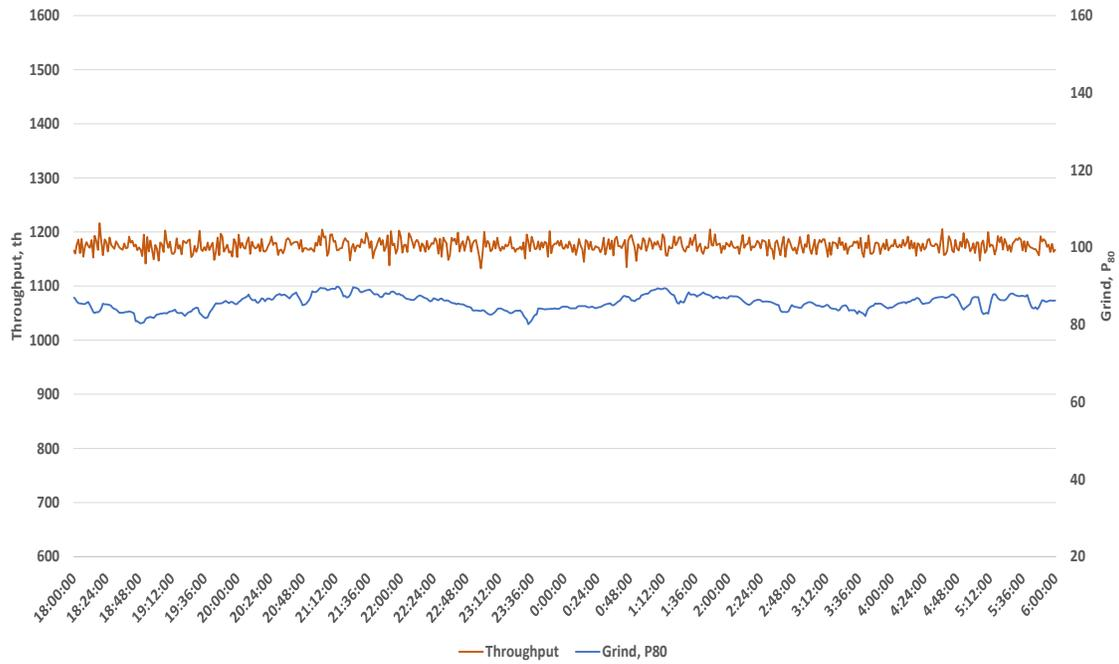
Figure 7—24-hour Throughput and Grind Trends for Tropicana
