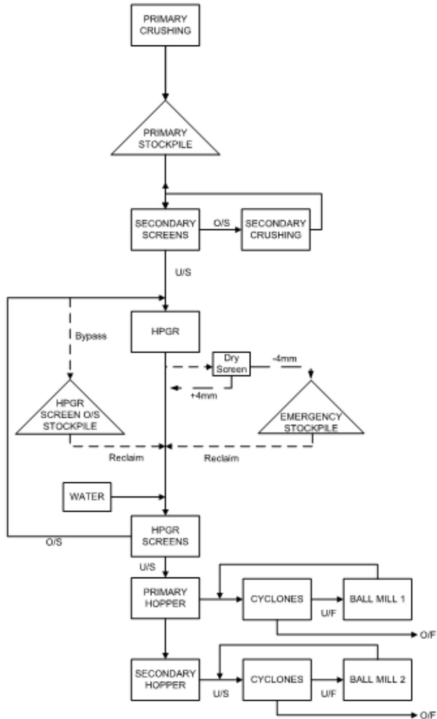
Figure 2—Tropicana Comminution Circuit Block Flow Diagram
