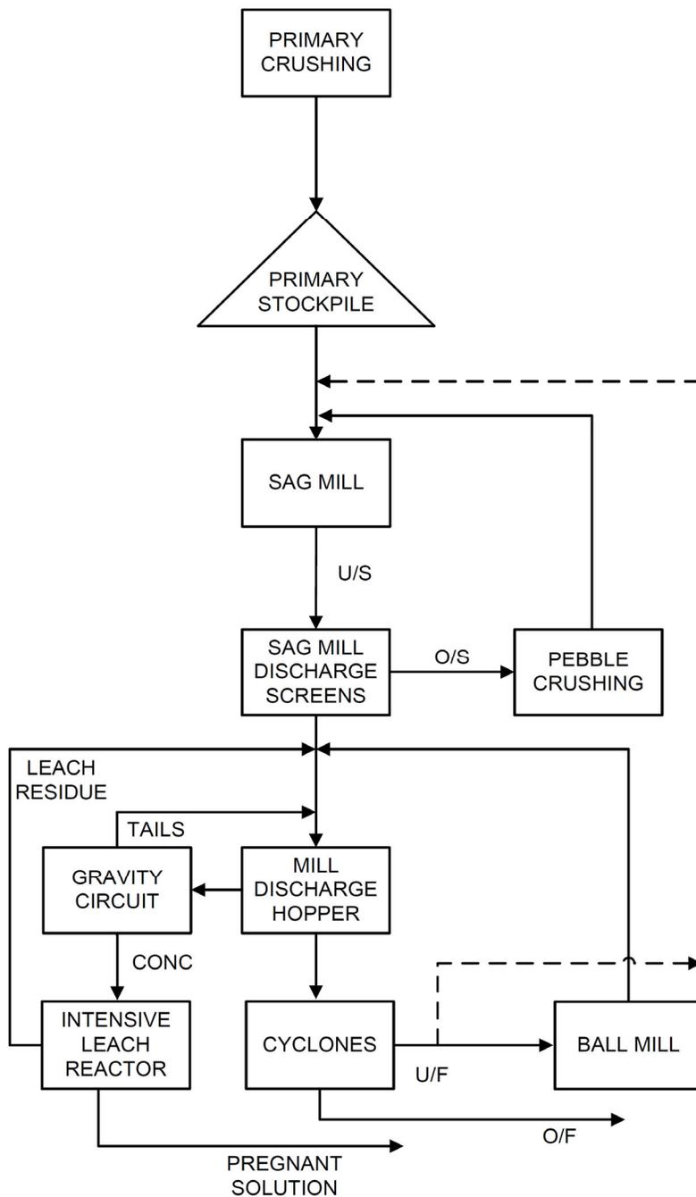
Figure 4—Gruyere Comminution Circuit Block Flow Diagram
