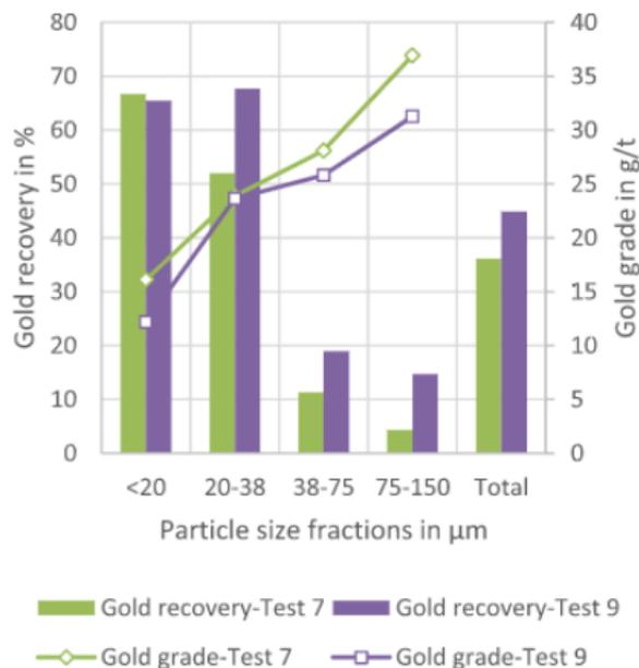
FIG 6 – Imhoflot pilot G-cell Au recovery by size and concentrate grade with optimised reagent addition (reproduced from Hoang et. al, 2022)
