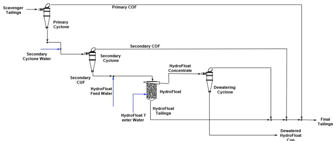
FIG 7 – Coarse Particle Flotation Limn Flowsheet
