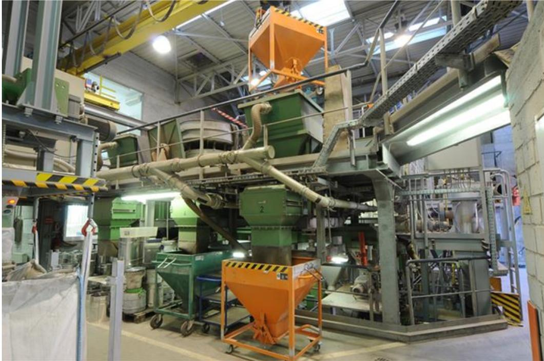
Figure 19: Continuous VRM and Grit Magnetic Separation Pilot Plant
