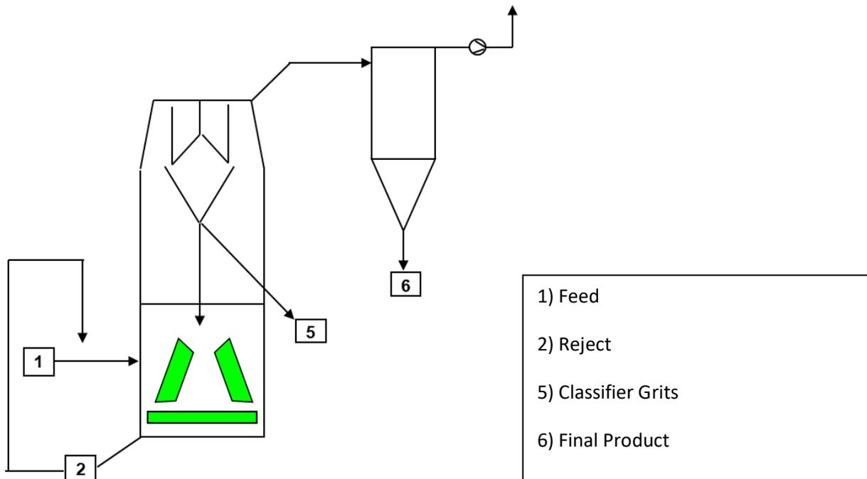
Figure 13: VRM Test Flowsheet with Optional Grit Extraction
