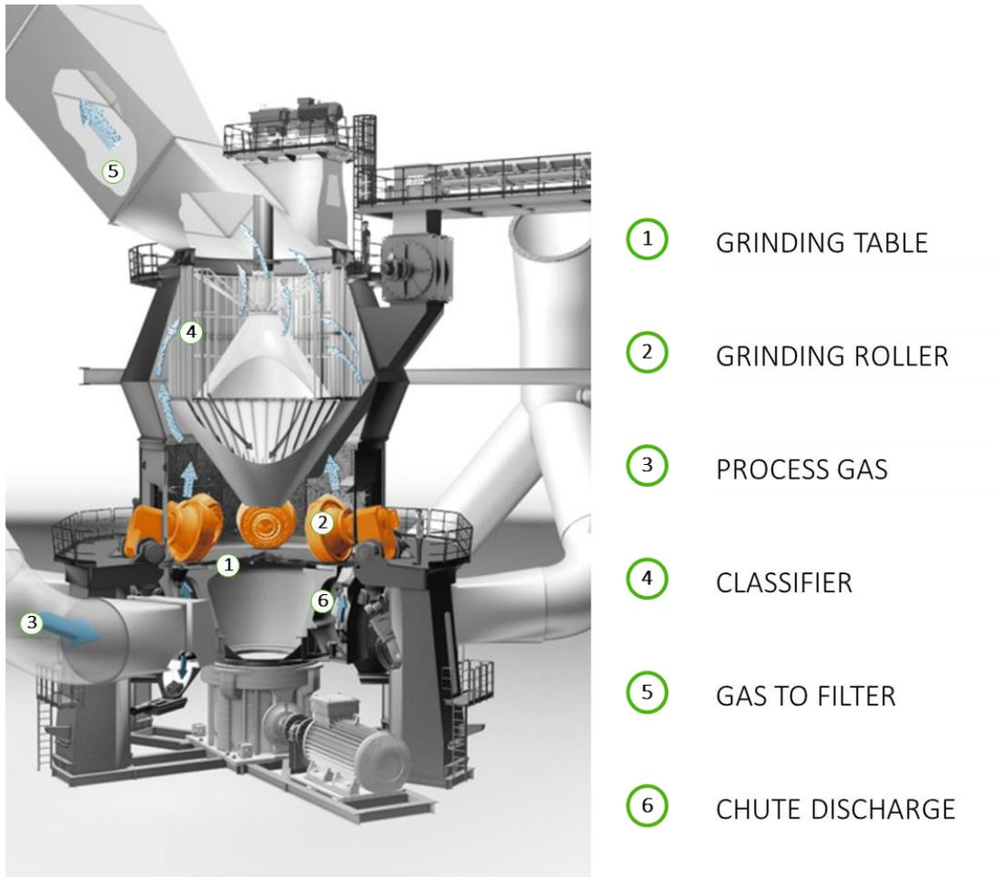
Figure 4: Schematic Loesche vertical roller mill
