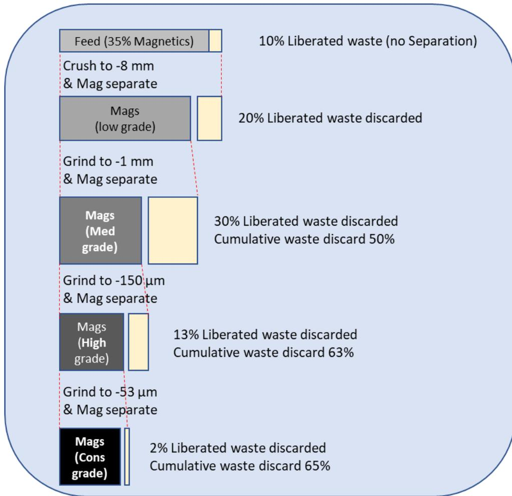
Figure 9: Progressive Comminution and Magnetic Separation Example for Magnetite
