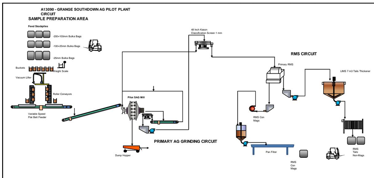
Figure 10: ALS Pilot AG Milling Flowsheet
