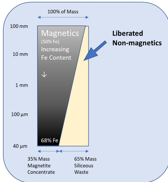
Figure 8: Conceptual Liberation of Waste from Magnetite Ore
