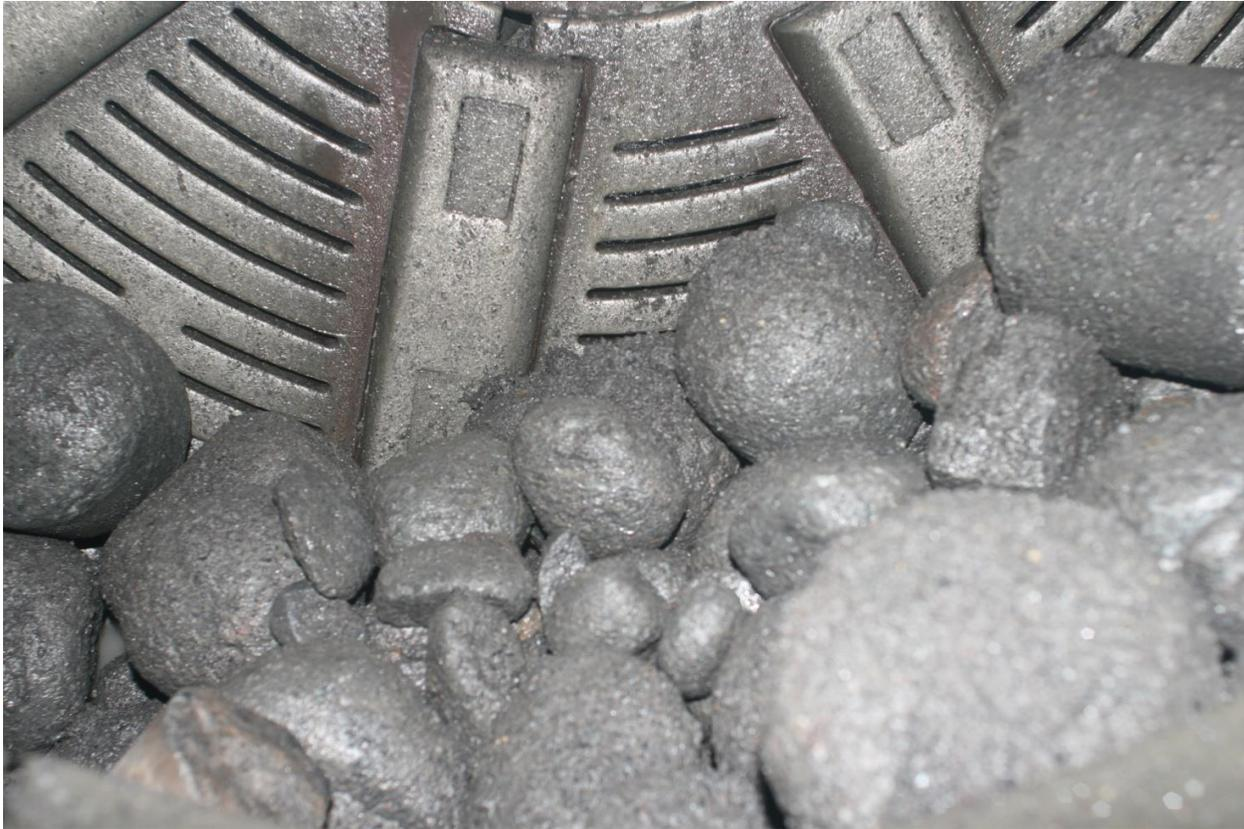
**Figure 11: AG Mill Charge showing Rounded Media**
