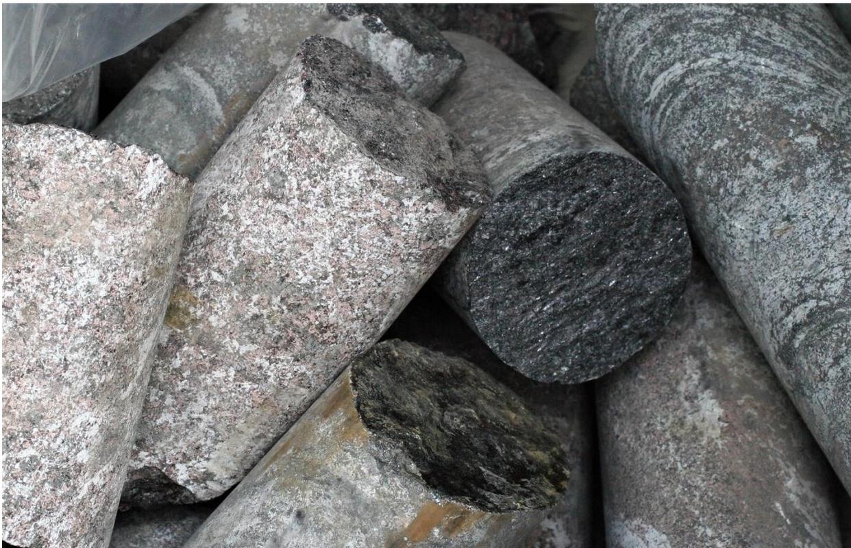
Figure 7: 150 mm Diamond Core for Metallurgical Testwork
