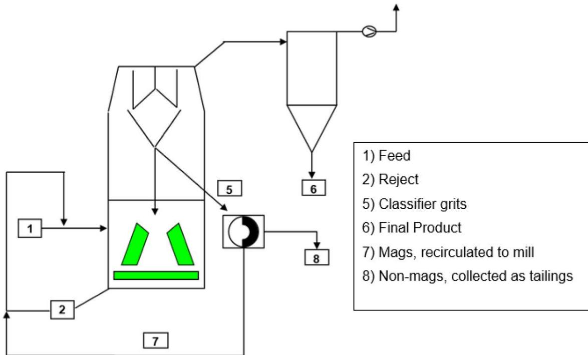
Figure 18: Continuous VRM and Grit Magnetic Separation Pilot Plant Flowsheet
