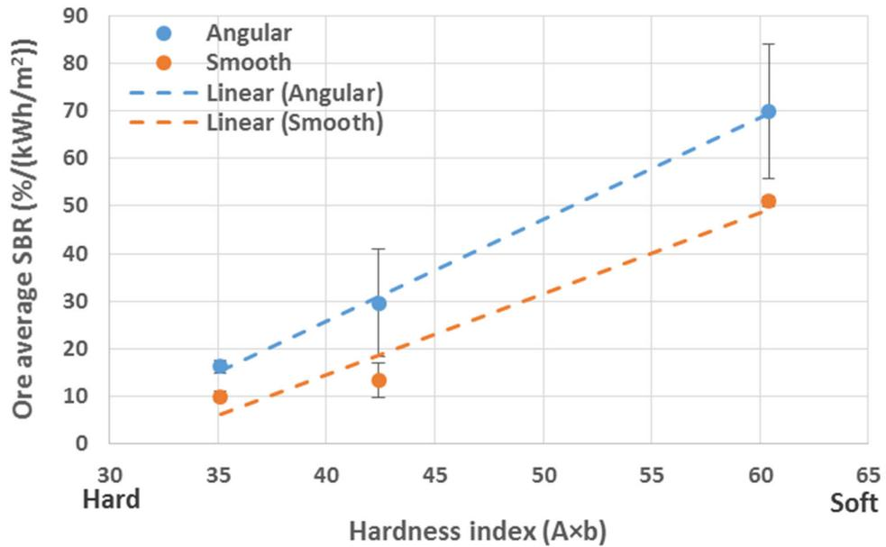
Figure 10—Relationship between SBR and ore hardness index (Axb) (Yahyaei, Weerasekara and Powell, 2015)
