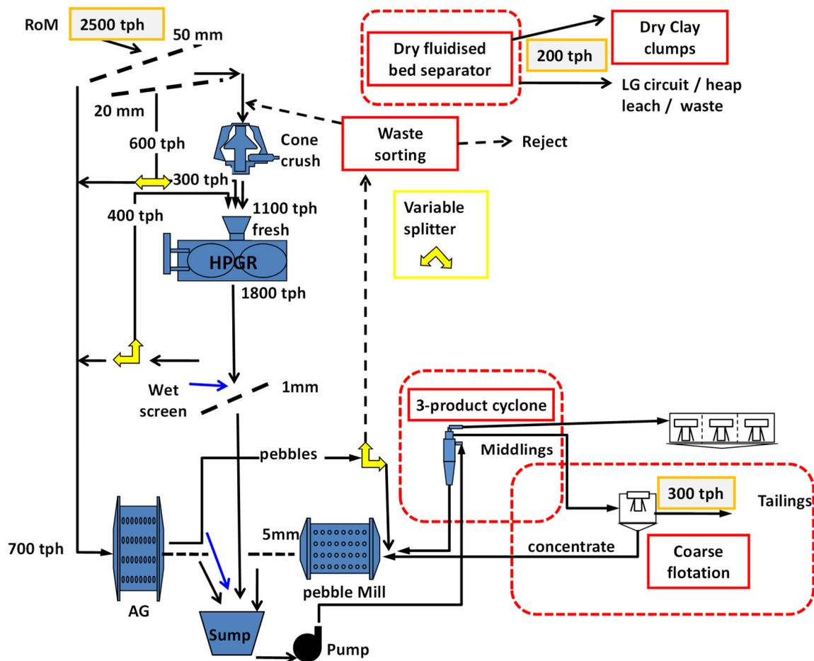
Figure 15—Flexi-circuit with AG mill, HPGR and future ore rejection options (Powell, 2013)
