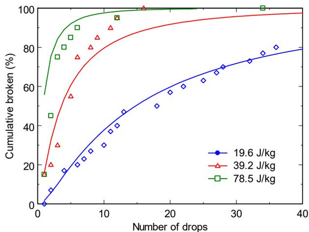
Figure 9—Cumulative breakage of 125-75 mm copper ore rocks from drop tests (Carvalho & Tavares, 2011).
