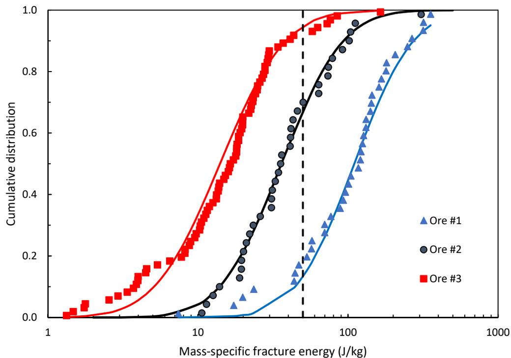
Figure 12—Distributions of fracture energies of particles of three iron ores in the size range 212-150 mm
