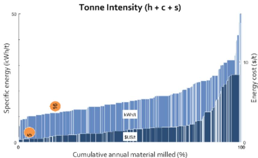
Figure 1—Aitik Energy curve benchmarking (Ballantyne, 2018)
