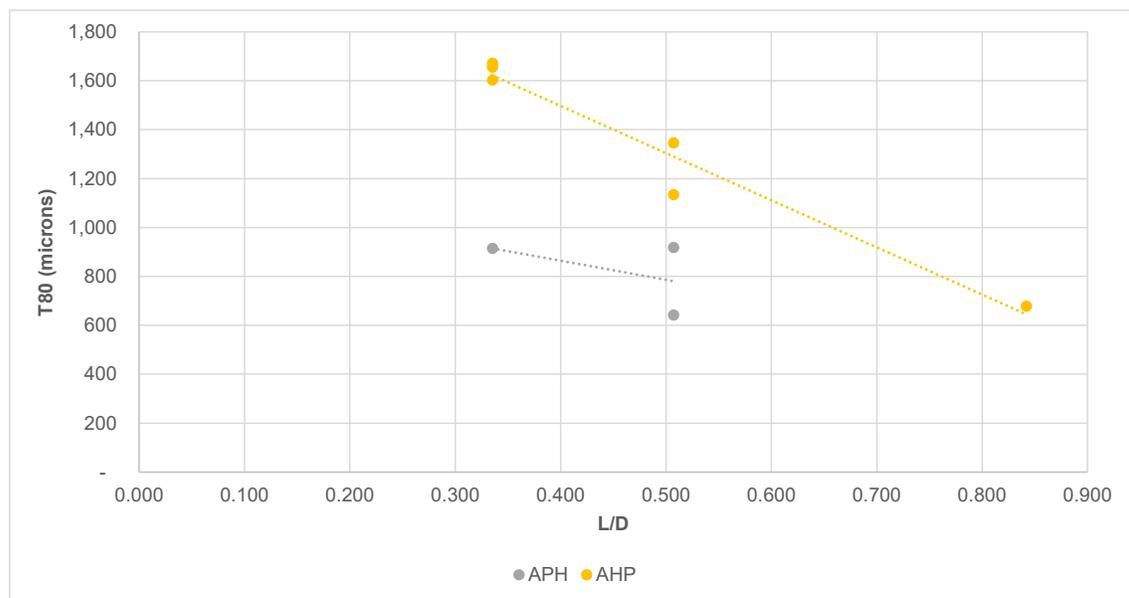
Figure 5—Impact of L/D on Transfer Size
