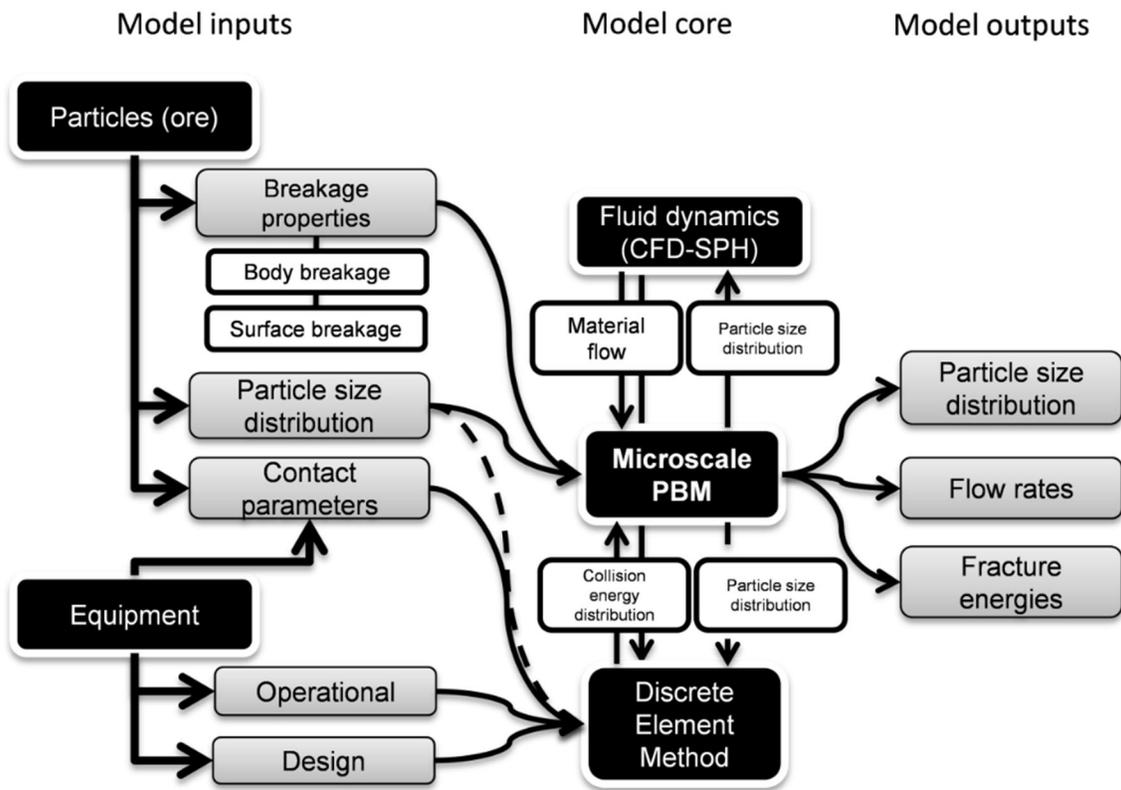
Figure 7—Mechanistic AG mill model structure (Carvalho and Tavares, 2011)
