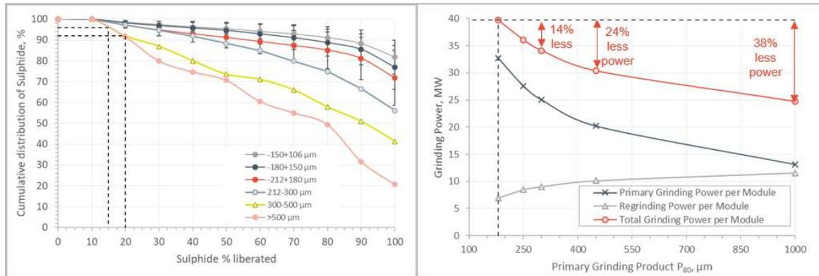
FIG 8 - Cumulative distribution of sulphides (covellite, enargite and pyrite) by degree of liberation (left), and simulated grinding power as a function of primary grinding product P80 (right).
