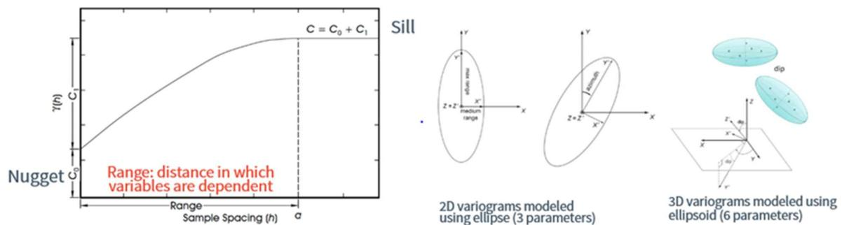
FIG 2 - Estimating 3D variability with geostatistics
