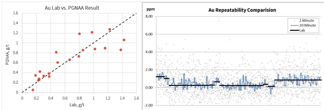
FIG 14 - PGNAA sensor vs. lab measurement (left) and repeatability (right)
