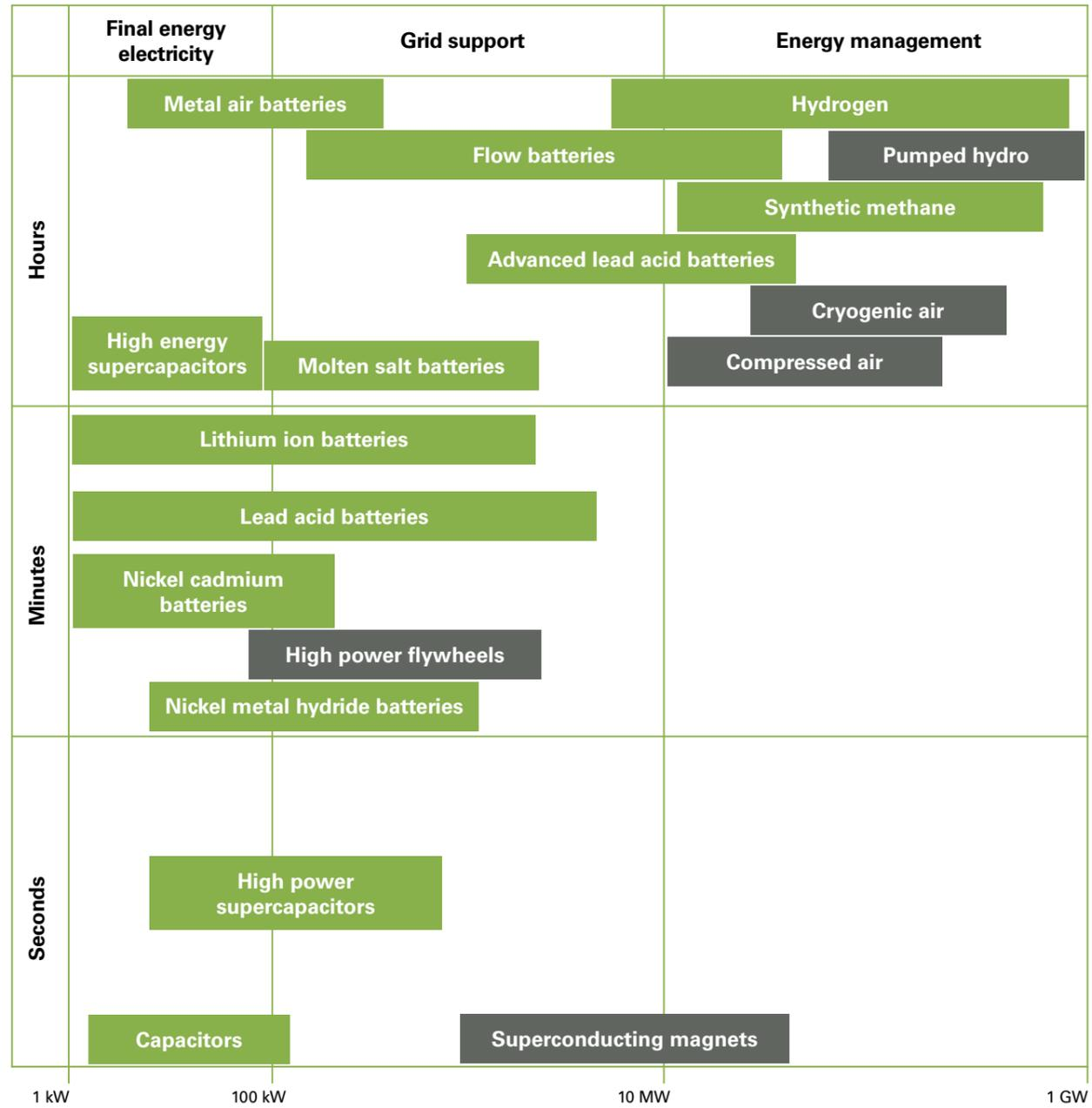
The figure above shows the size (on the horizontal) and the discharge time (on the vertical) that is ideal for different energy storage technologies. Pumped hydro could show some promise for mining operations as the height difference between the bottom and top of a pit, between two pits or using a mine shaft could potentially be utilised to store energy.
