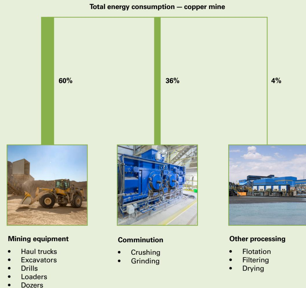
Figure 1 – High level energy consumption: copper mine
