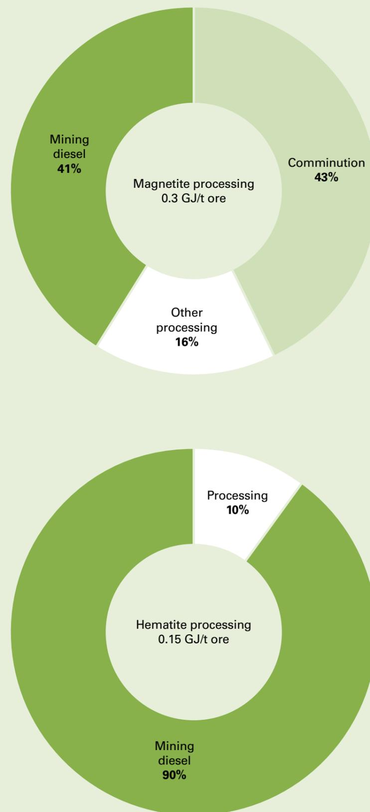
Figure 12—Split of energy for iron ore processing
