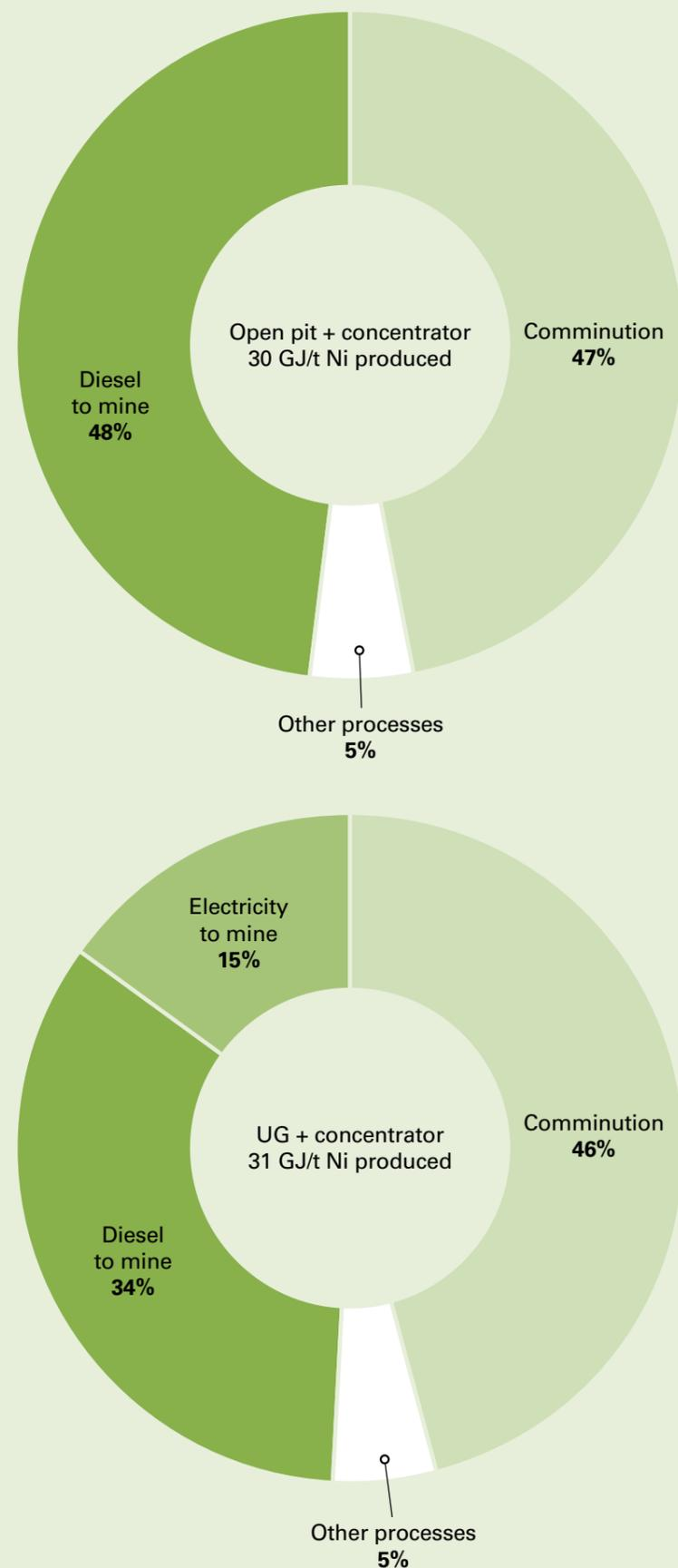
Figure 10—Split of energy consumption for nickel sulphide concentrators
