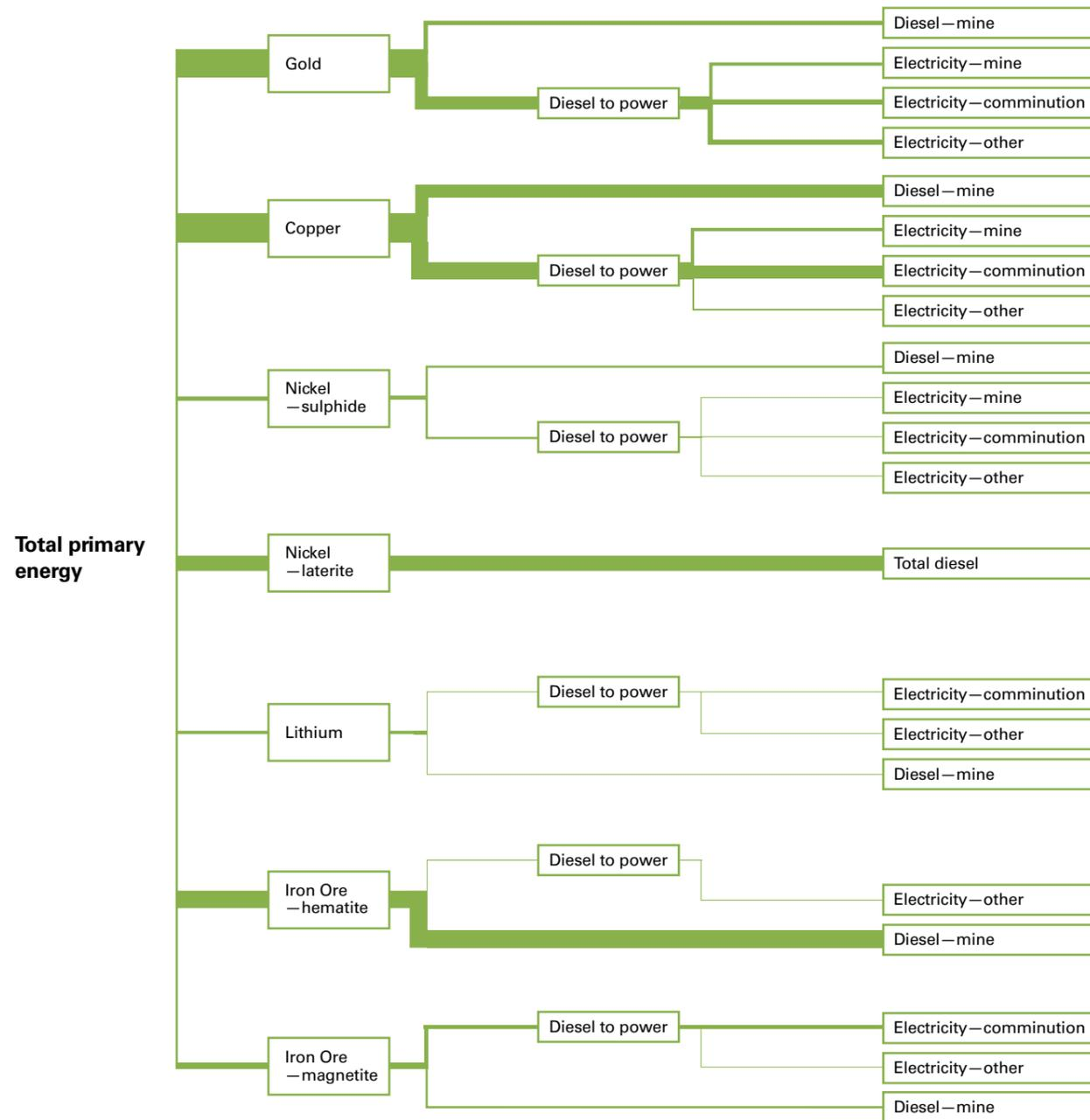
Figure 4 – Sankey diagram showing energy flows in mining
