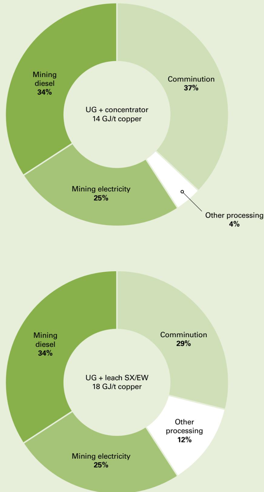
Figure 9—Split of energy consumption in copper underground operations
