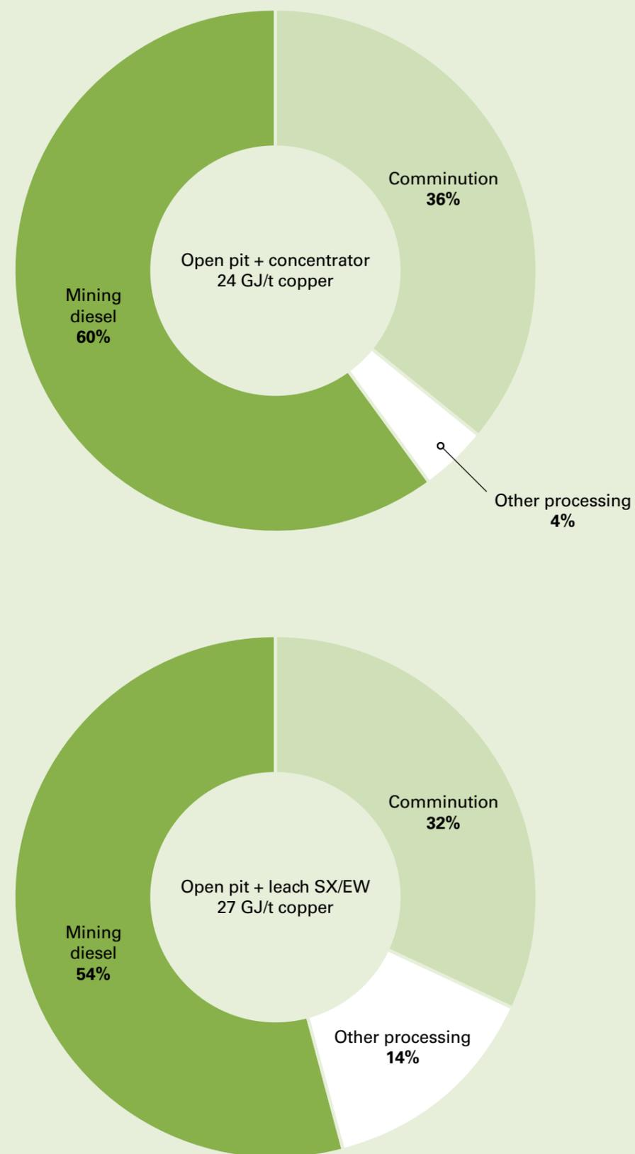
Figure 8—Split of energy consumption in copper open pit operations
