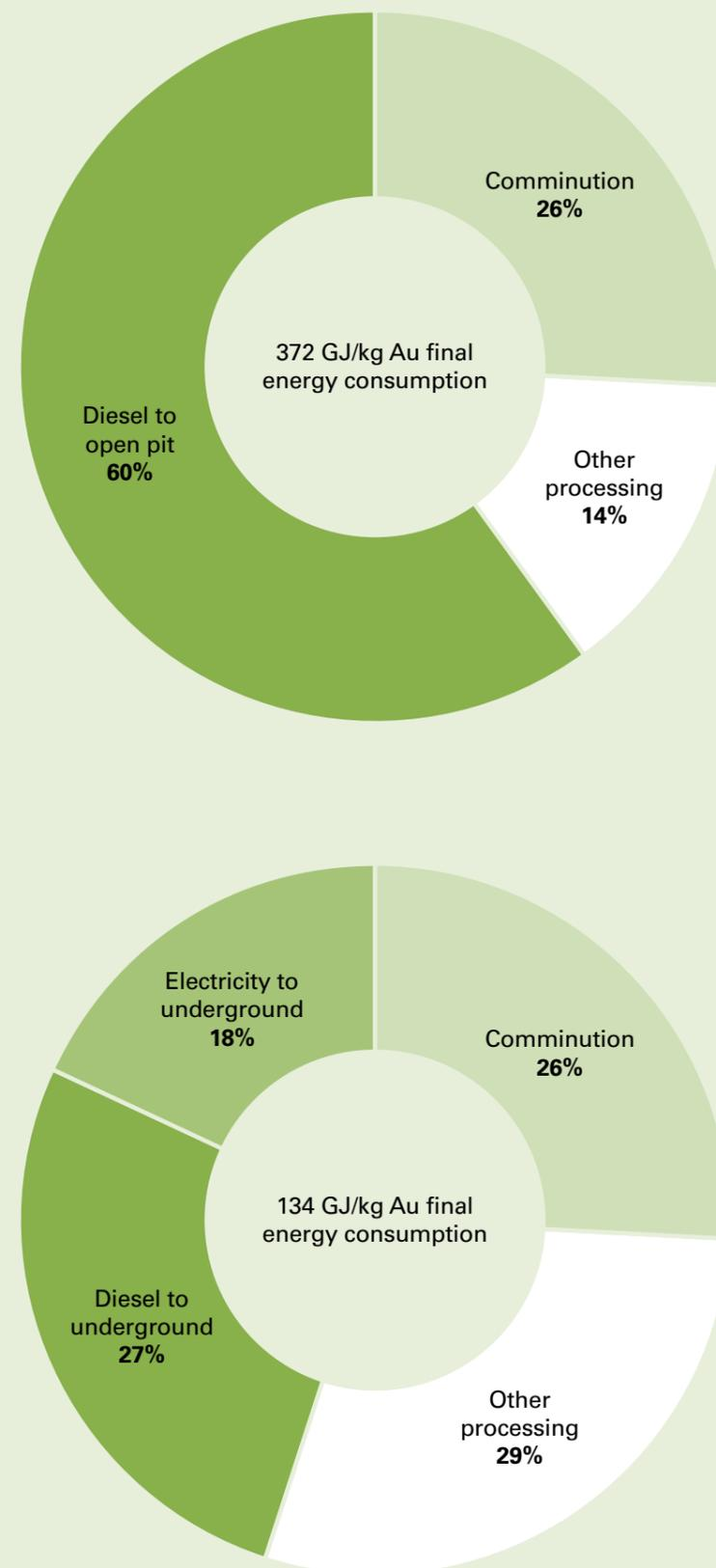
Figure 11 — Split of energy consumption for gold operations (open pit: top, underground: bottom)
