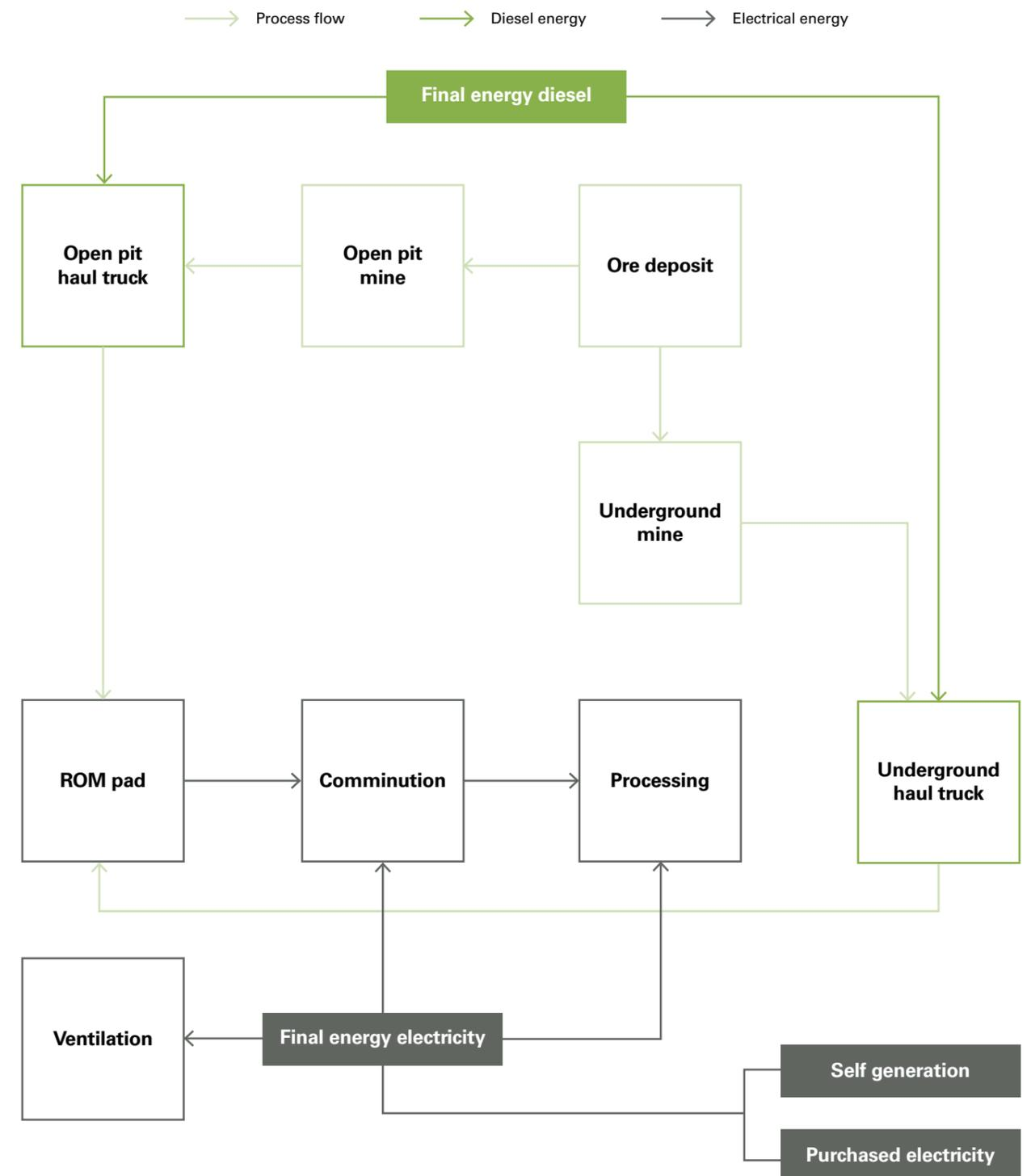
Figure 7— General flowchart of a mining operation showing key energy users
