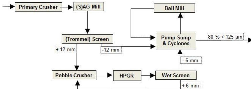
Figure 3. Penasquito Flow Sheet around HPGR.
