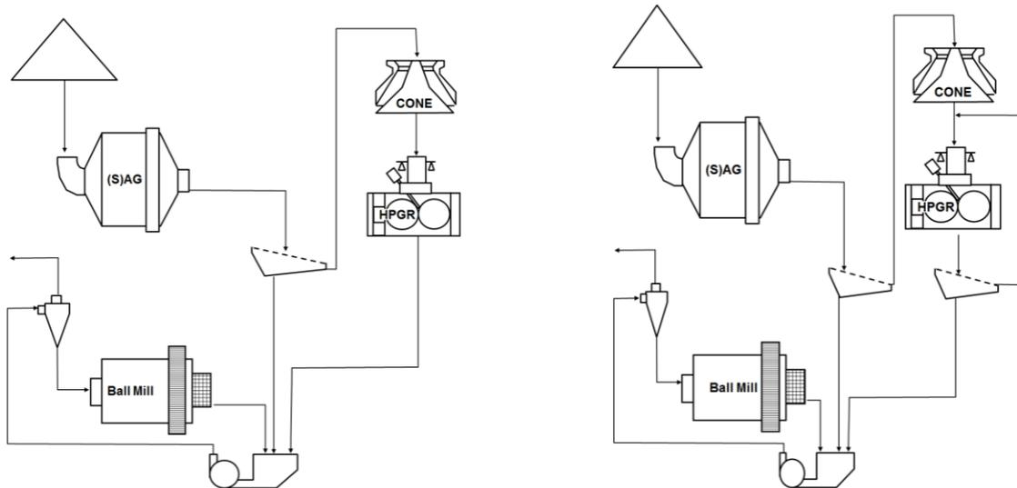
Figure 7 (left side). Pebble crushing by cone and subsequent HPGR in open circuit, product forwarded to downstream ball mill discharge pump sump.
