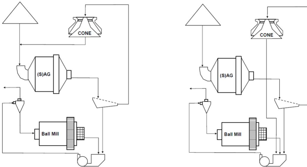
Figure 5 (left side). Pebble crushing by Cone crusher, product back to (S)AG.
