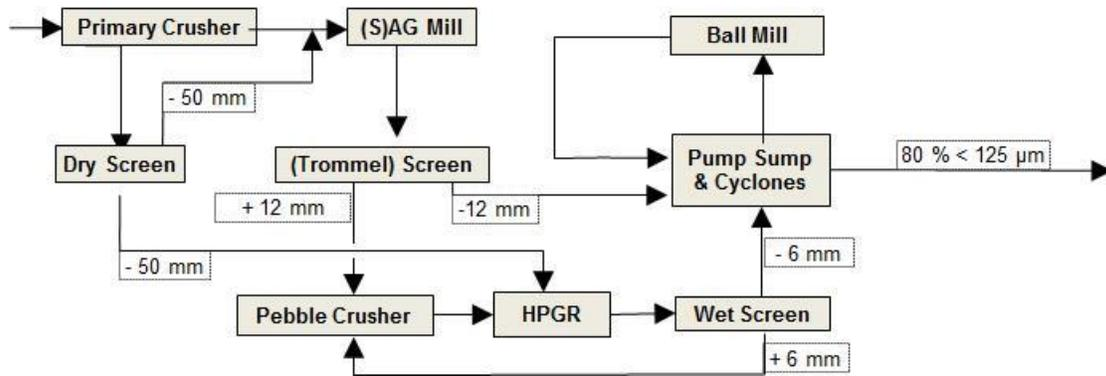
Figure 4. Penasquito Flow Sheet around HPGR, adapted.
