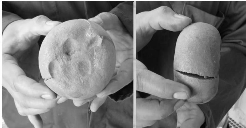
Figure 1. Example of Aerofall ball retrieved after HPGR passage, cracked and dented by HPGR rolls.
