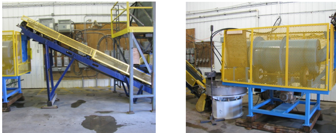
Figure 6 - Scrubbing Equipment at SGS Lakefield
