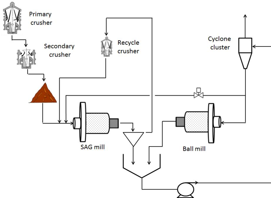
Figure 1 - Sulphide Circuit flow diagram
