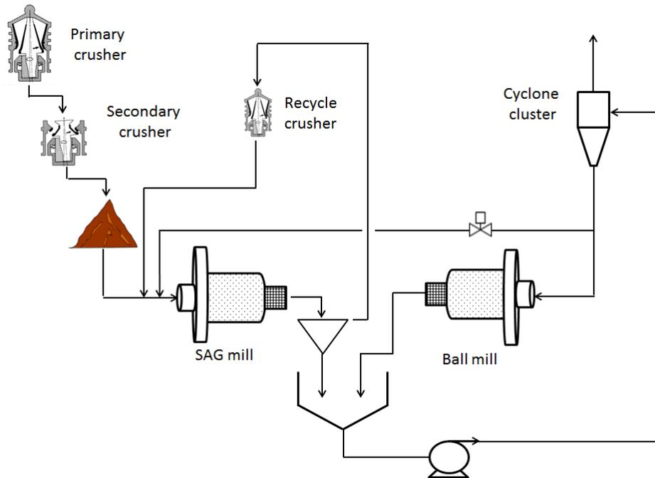
Figure 1 - Sulphide Circuit flow diagram
