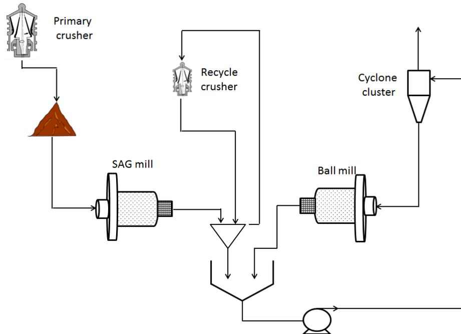
Figure 3 - Oxide Circuit flow diagram
