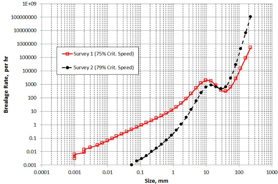
Figure 6 - Breakage rates for the Oxide SAG mill from the survey data showing the effect of mill speed
