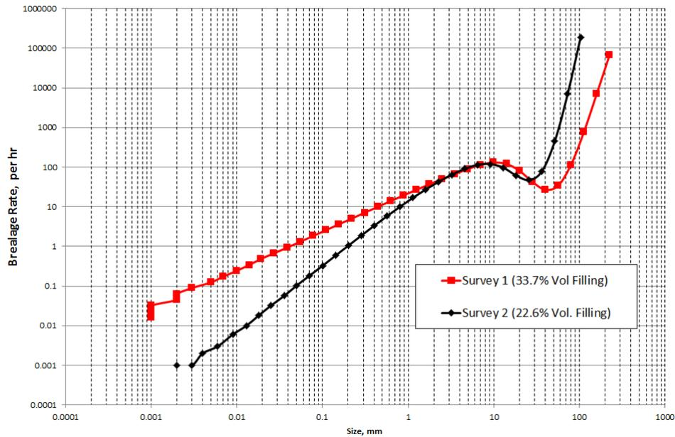
Figure 4 - Breakage rates for the Sulphide SAG mill from the survey data
