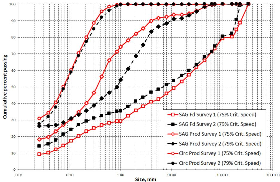
Figure 5 - Comparison of particle size distributions of the oxide circuit surveys
