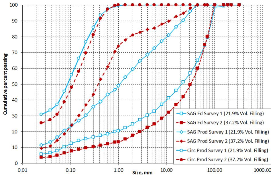
Figure 7 - Comparison of particle size distributions of some key streams in the mixed circuit surveys
