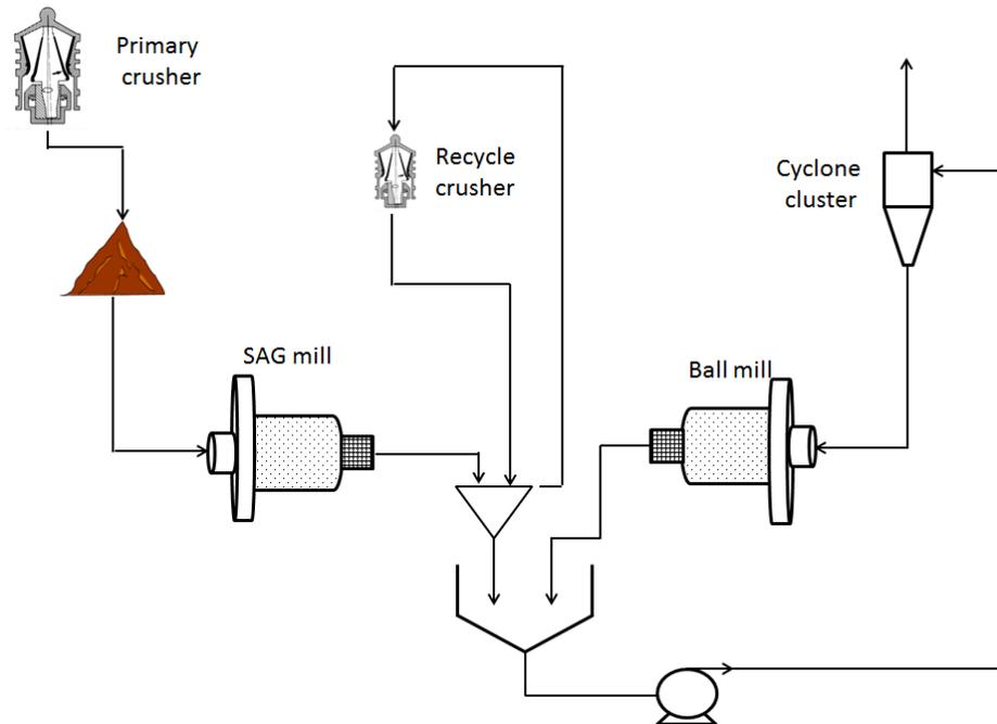
Figure 3 - Oxide Circuit flow diagram
