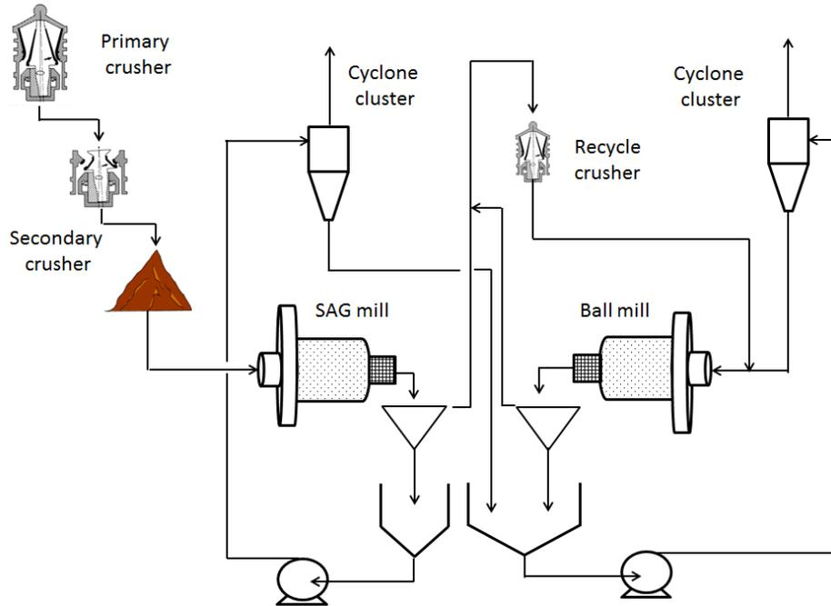
Figure 2 - Mixed Circuit flow diagram
