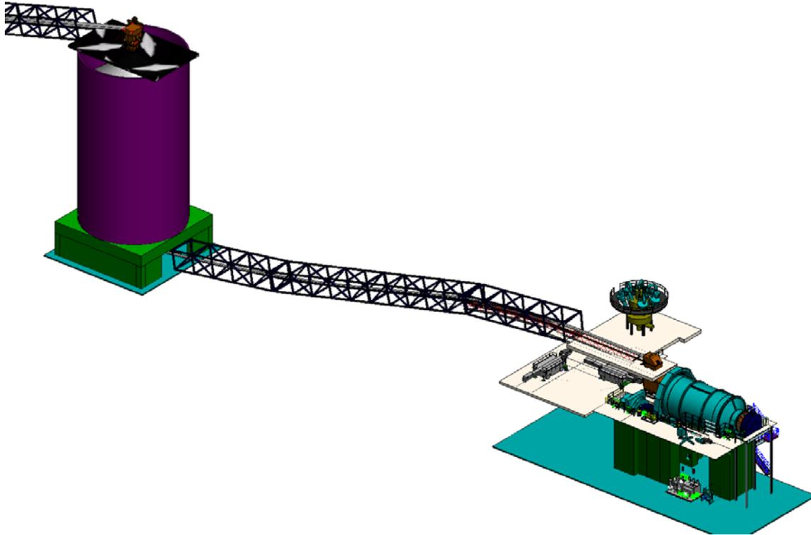
Figure 16 – Project #2 Base Case fine ore bin and grinding circuit 3D model
