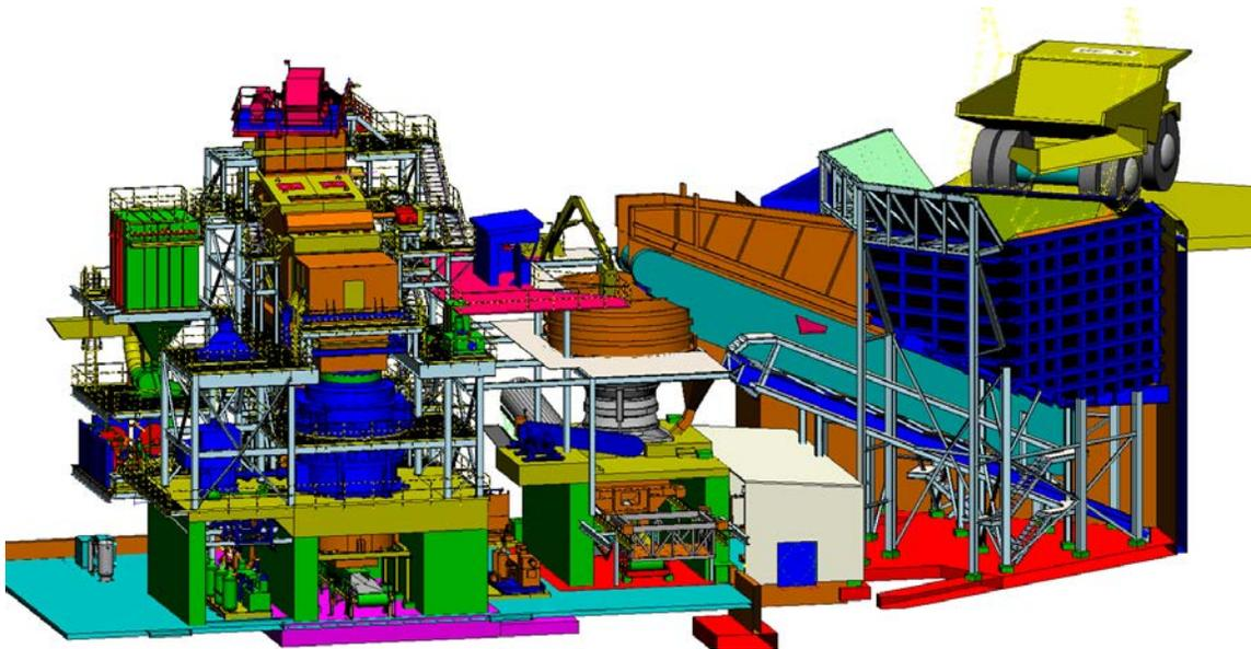
Figure 12 – Project #1 Alternative primary and secondary crushing circuit 3D model
