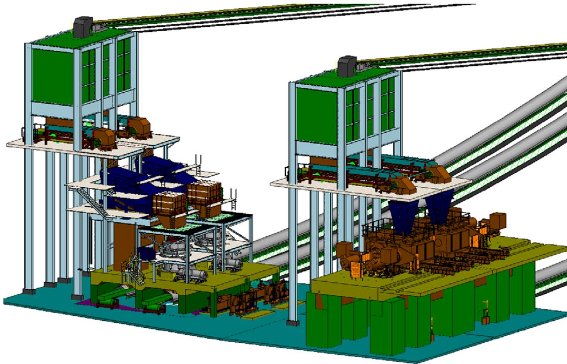
Figure 9 – Project #1 Base Case secondary crushing and HPGR circuit 3D model
