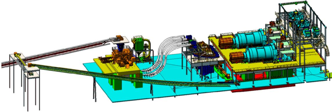
Figure 13 – Project #1 Alternative HPGR and grinding circuit 3D model
