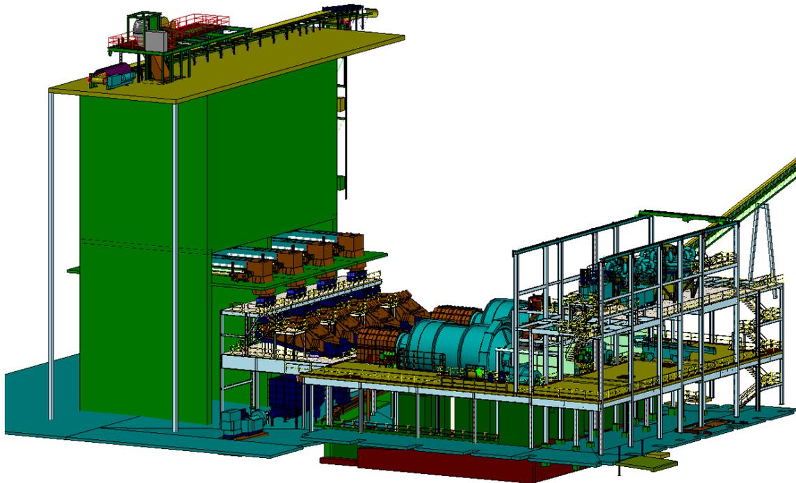
Figure 10 – Project #1 Base Case grinding circuit 3D model
