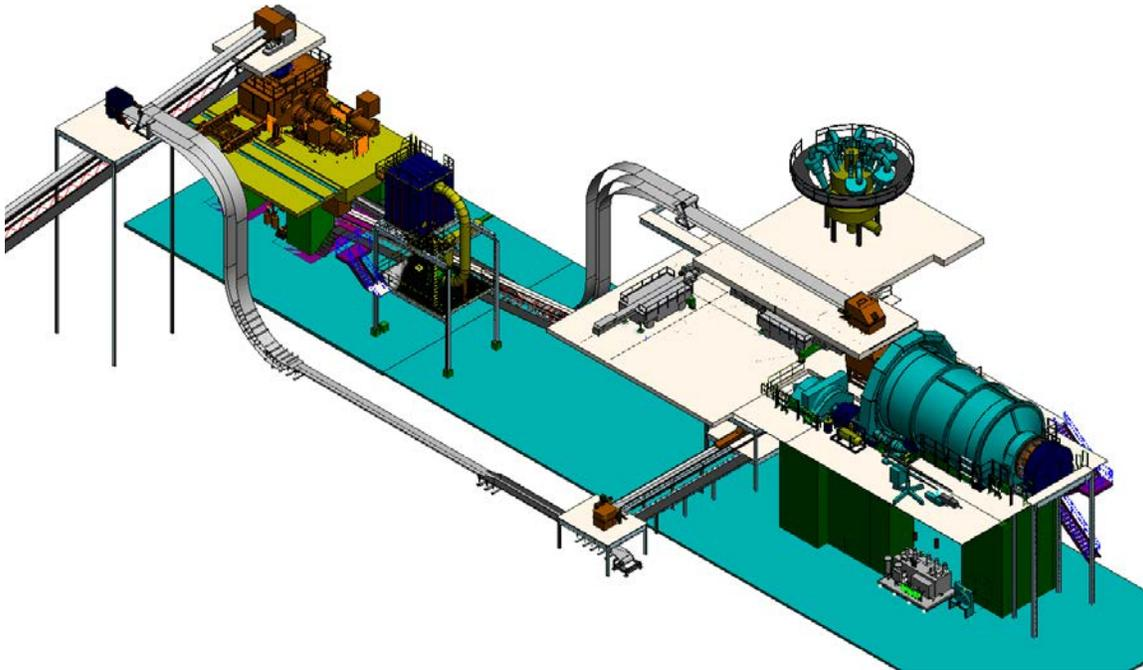
Figure 19 – Project #2 Alternative HPGR and grinding circuit 3D model
