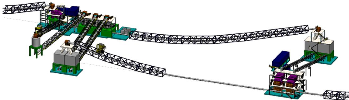
Figure 15 – Project #2 Base Case secondary and tertiary crushing circuit 3D model
