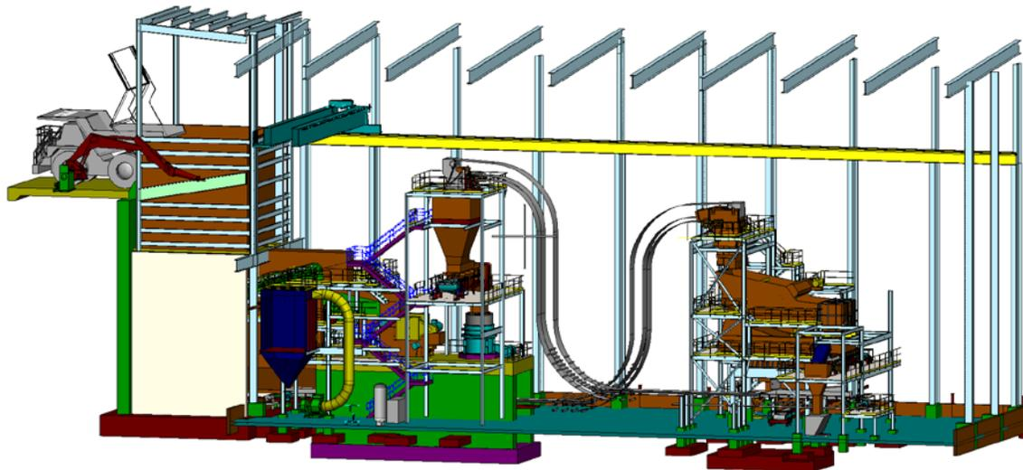
Figure 18 – Project #2 Alternative primary and secondary crushing circuit 3D model
