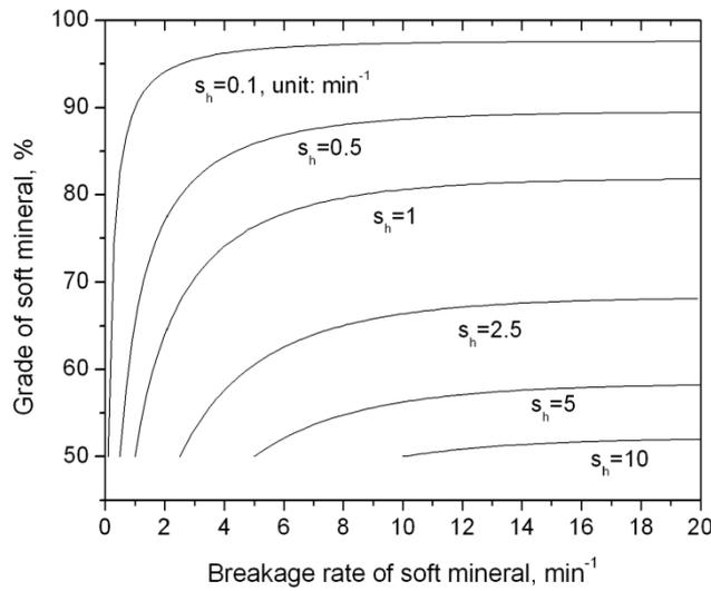
Figure 6 – Effect of breakage rates on the grade of soft mineral in the product: grinding time 0.25 min,
