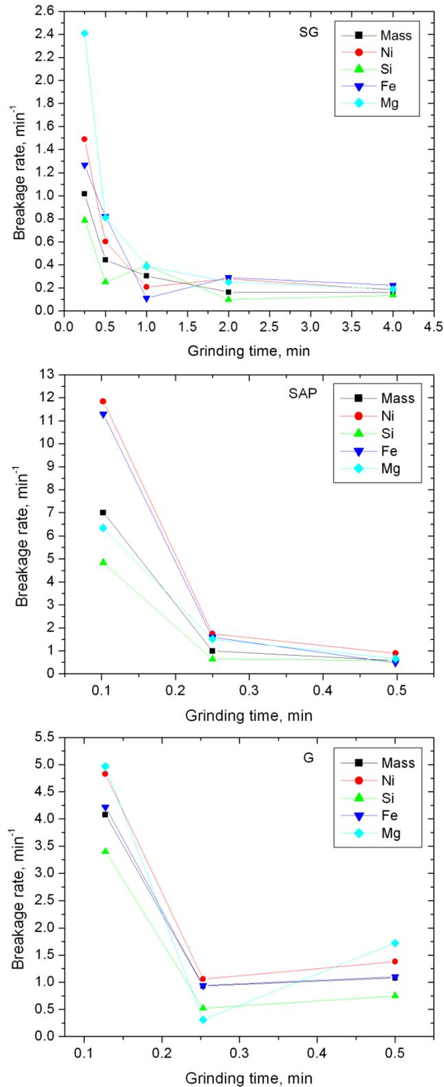
Figure 5 – Effect of grinding time on the rate of breakage of nickel laterites
