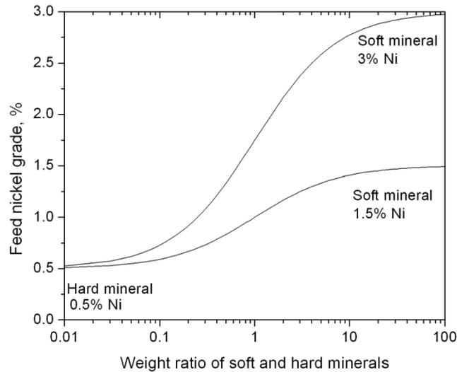
Figure 9 – Effect of nickel distribution on the feed nickel grade
