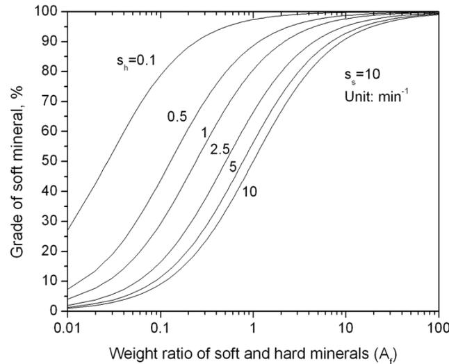
Figure 8 – Effect of minerals weight ratio on the grade of soft mineral in the screen undersize product
