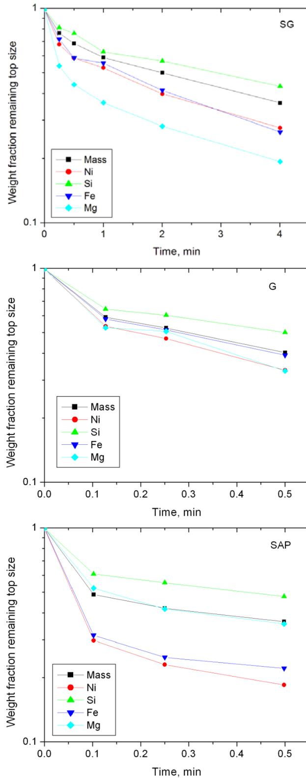
Figure 1 – Grinding behaviour with respect to the sample mass and various elements
