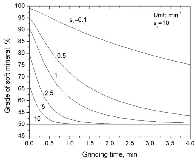
Figure 4 – Effect of grinding time on the grade of soft mineral in the screen undersize product
