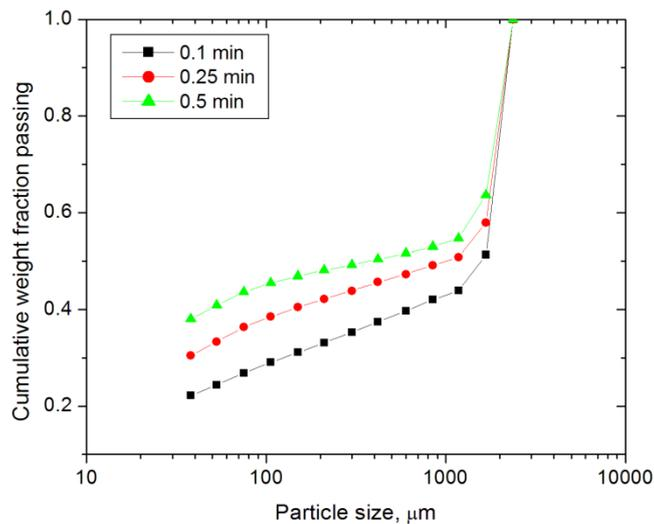
Figure 2 – Particle size distribution of the SAP nickel laterite grinding product: feed size 2.38-1.68 mm
