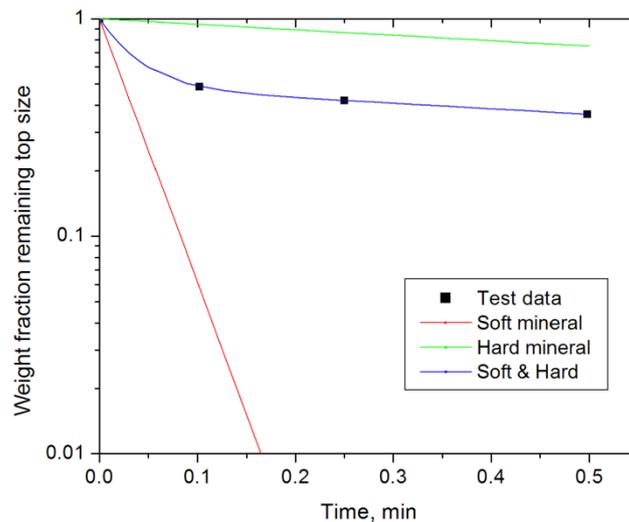
Figure 3 – Grinding behavior with respect to sample mass: SAP nickel laterite, assume the feed composed of soft and hard minerals, feed size 2.38-1.68 mm
