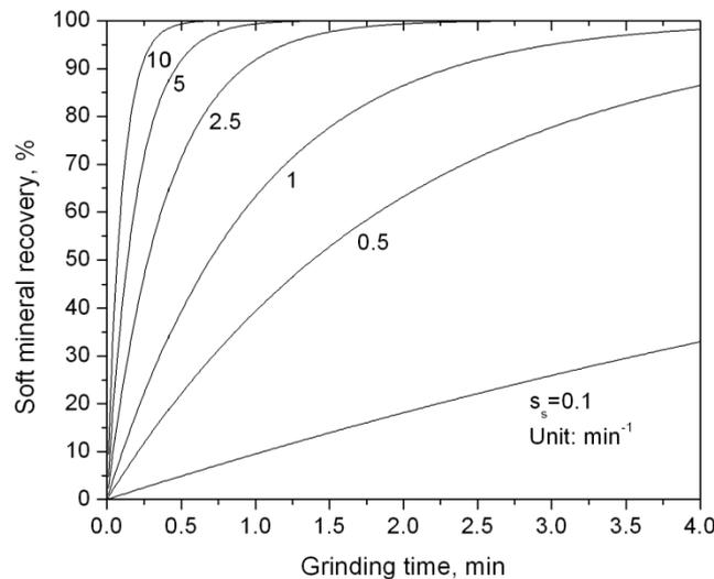
Figure 7 – Effect of grinding time on the soft mineral recovery
