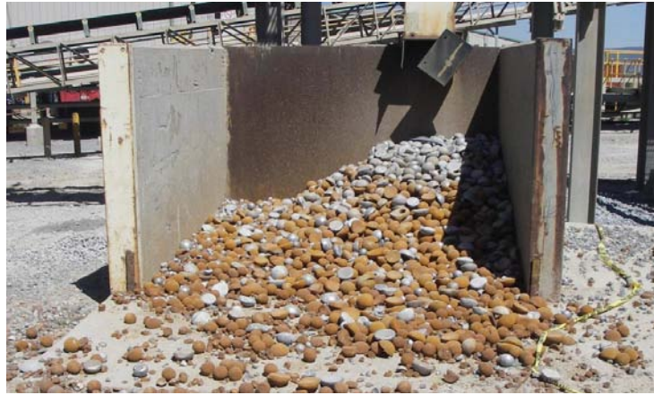
Figure 7 – North Mara SAG mill reject steel
