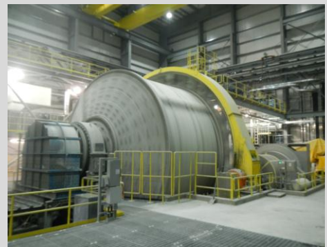
The 7,500-HP SAG mill operates in the grinding circuit.
