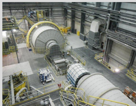
The grinding circuit mills break solid material into smaller pieces.
