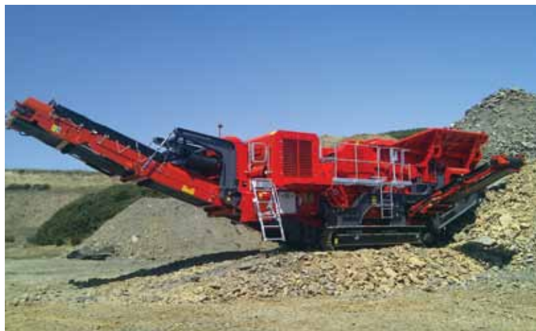
Hillhead 2012: The Terex Finlay J-1175 tracked mobile jaw crusher can be powered by either a Tier 3/Stage 3A Caterpillar C9 or a Tier 4i Scania DC970A engine used with hydrostatic transmission.
