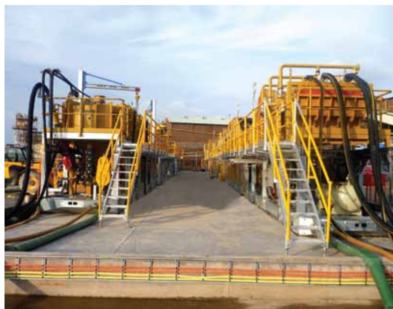
The Gekko Python 500 modular plant at the Gold Fields Kloof Growth project uses InLine pressure jigs to reject gangue from vertical shaft impact crusher product, eliminating ball milling and reducing comminution energy consumption.
