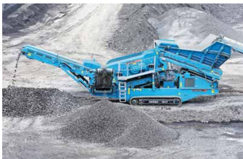
Powerscreen says the new Warrior 1400X screening plant can be equipped with a Tier 3/Stage 3A or Tier 4i/Stage 3B Caterpillar engine. Using reduced running speed and enhanced hydraulics the 1400X offers up to a 15% reduction in fuel consumption compared with its predecessor.
