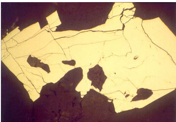
Fig. 6 Cross section of a sulfide particle in ore treated by HPGR showing the micro-fractures in the sulfide particle that would accelerate bio-oxidation. Source: Baum (1997).
