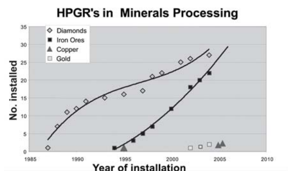
Fig 1. Growth in HPGR applications in diamond iron ore, copper and gold ore processing. Source: Knecht (2004)
