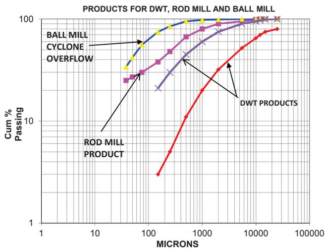
FIG 10 - JKDWT, DWT, rod mill and ball mill cyclone product slopes.
