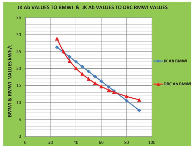
FIG 3 - Conversion of JK Ab to Bond ball mill work index values and JK Ab to DB Consulting Bond rod mill work index values.
