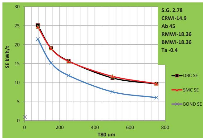
FIG 7 - Bond SE versus DB Consulting and SMC drop weight index autogenous/semi-autogenous specific energies from T80s of 75 µm to 750 µm based on the input parameters shown on the graph.
