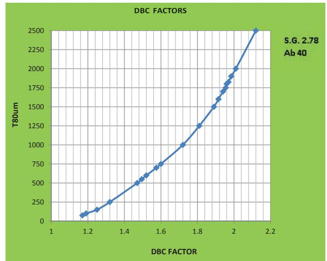
FIG 2 - Autogenous/semi-autogenous DB Consulting factors for material with a specific gravity of 2.78 and an Ab of 40.
