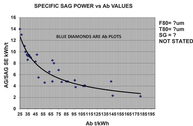
**FIG 12** - Ab versus autogenous/semi-autogenous grinding, SE trend curve.
