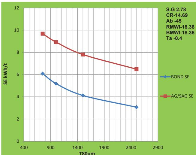
FIG 5 - Bond SE versus DB Consulting autogenous/semi-autogenous specific energy for T80s of 2500 µm to 750 µm based on the input parameters shown on the graph.
