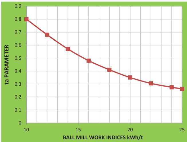
FIG 4 - Conversion of ta values to Bond ball mill work index values.
