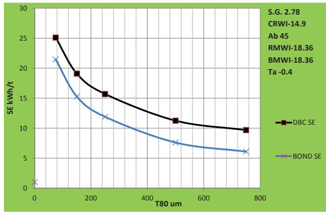
FIG 6 - Bond SE versus DB Consulting autogenous/semi-autogenous specific energy from T80s of 750 µm to 75 µm based on the input parameters shown on the graph.
