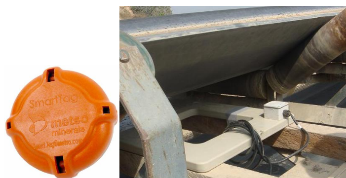
Figure 3: SmartTag™ RFID Ore Tracking Tag & Antenna Installation
