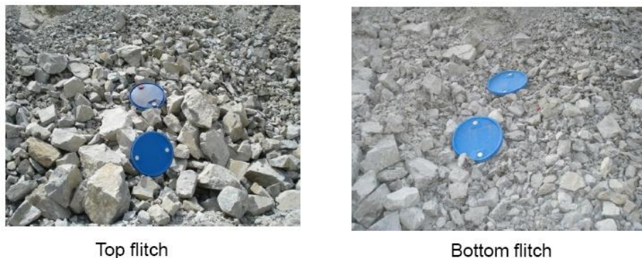
Figure 2: Example Blast Fragmentation from Top vs. Bottom Flitch (Double Benching)
