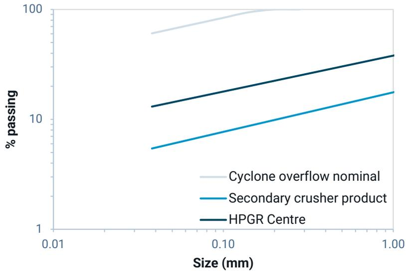
Figure 11 - Fractal Energy modelling output particle size distributions
