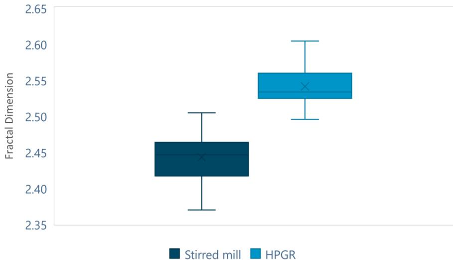
Figure 5 - Fractal dimension of breakage for stirred mills and HPGR
