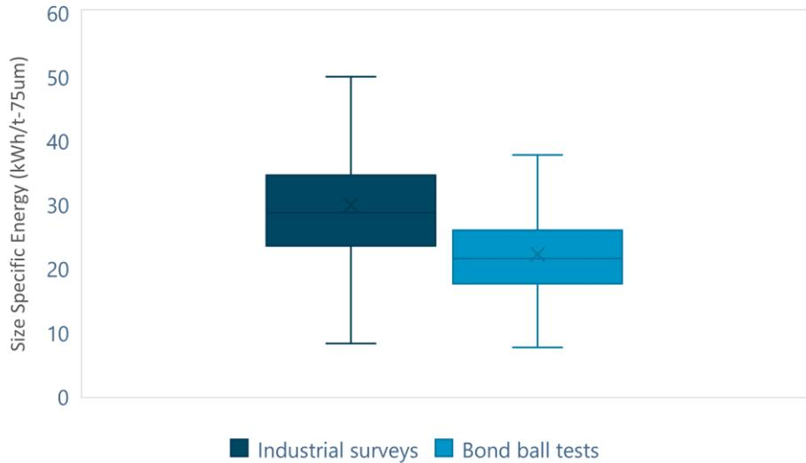
Figure 9 - Difference between SSE75 measured in the Bond ball mill test and measured in industrial surveys
