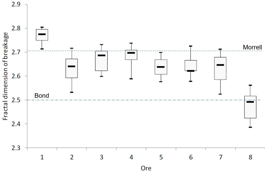
Figure 2 - Fractal dimension of breakage for 8 different ores displayed as a box-and-whisker plot highlighting the minimum, maximum, median and interquartile range. The Fractal dimension equivalent to Bond and Morrell are presented.
