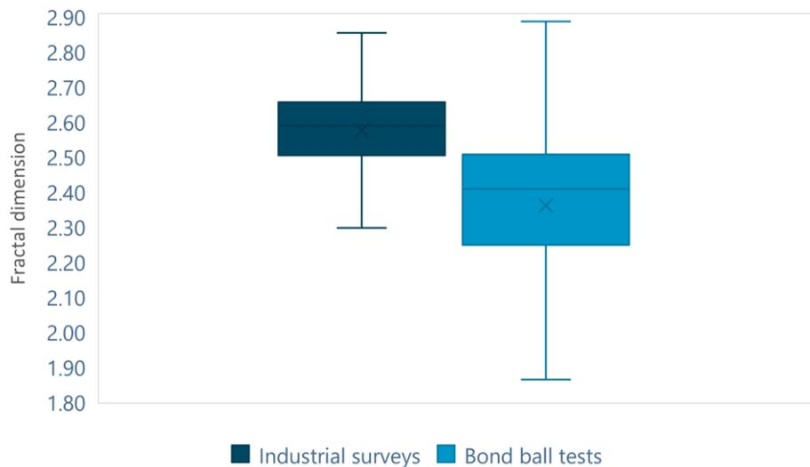
**Figure 8 - Fractal dimensions recorded from the Bond ball mill work index test in relation to the fractal dimensions of industrial surveys**
