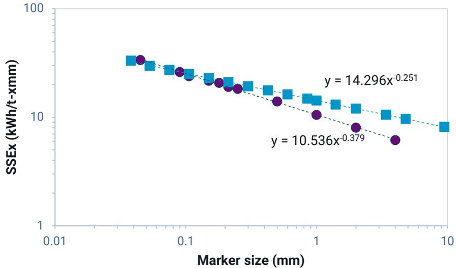
**Figure 10 - Fractal dimension of breakage analysis on HPGR testwork with edge recycle.**
