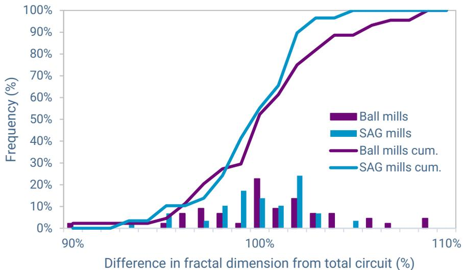
**Figure 4 - Distributions of the ratio in fractal dimension of breakage for SAG and ball mills in comparison to the total circuit**
