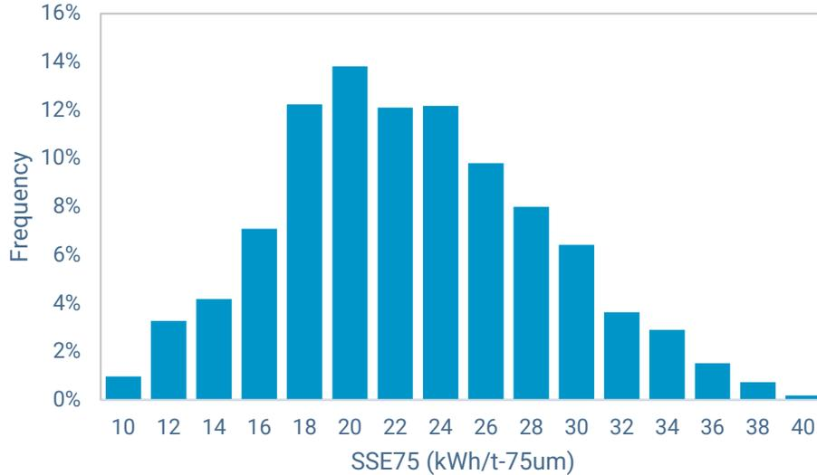
**Figure 6 - Distribution of SSE75 from Bond ball mill work index tests**
