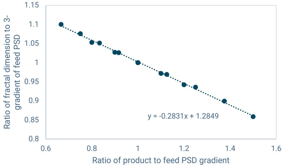
**Figure 12 - Fundamental relationship between the gradient of the feed and product size distributions and the fractal dimension of breakage**
