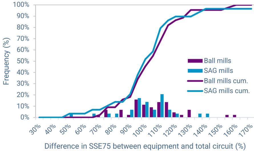
**Figure 3 - Distribution of the ratio of SSE75 for SAG and ball mills in comparison to the total circuit.**
