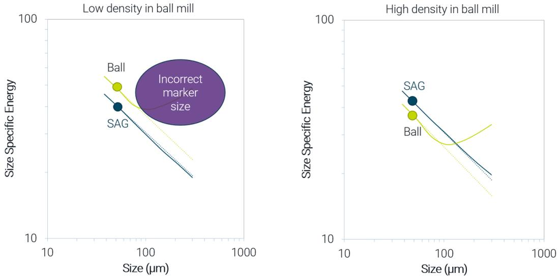
**Figure 1 - Examples of using SSE across a range of marker sizes and the impact of ball mill charge density (after Ballantyne, 2019)**
