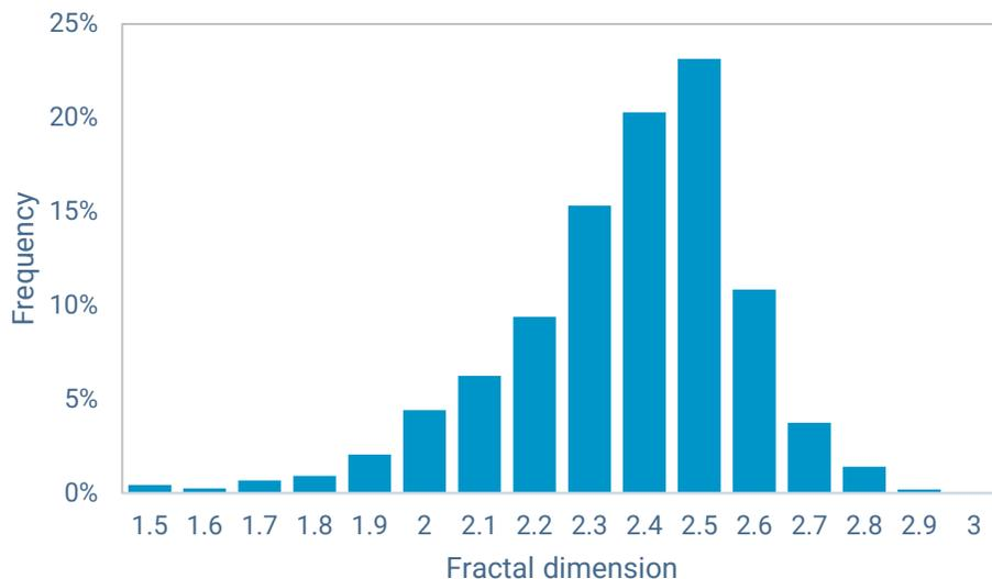
**Figure 7 - Distribution of fractal dimension from Bond ball mill work index tests**
